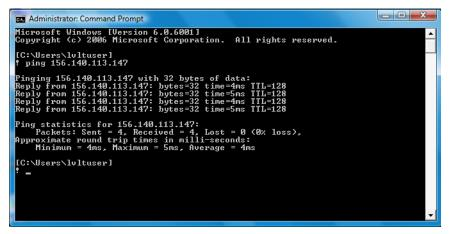
Figure 62 Example Using Ping Utility
