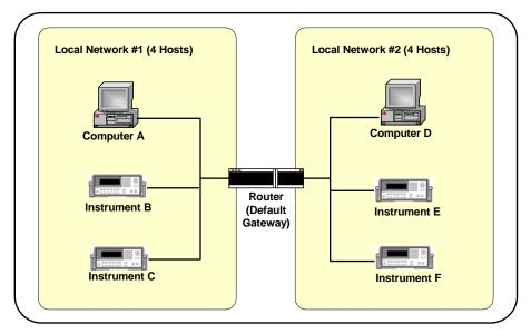
Figure 66 Two Networks (Subnets) Using a Router
