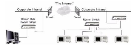
Figure 31 Internet access through firewall
