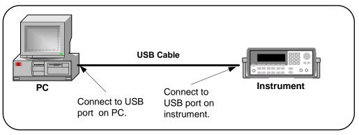
Figure 21 Typical USB Interface System
