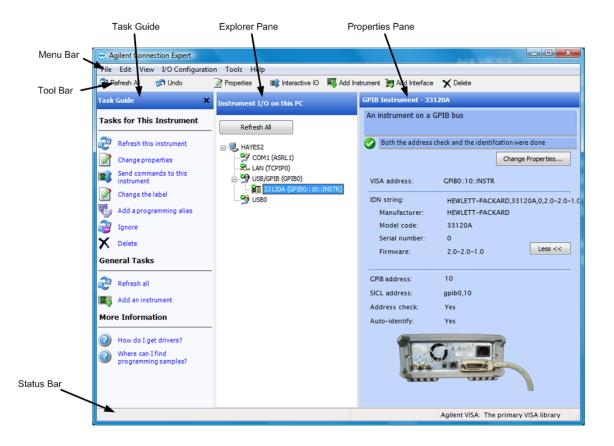
Figure 3 Agilent Connection Expert Screen
