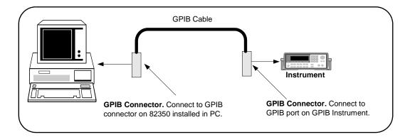
Figure 15 Connecting a Single GPIB Instrument
