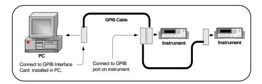
Figure 14 Typical GPIB Interface System
