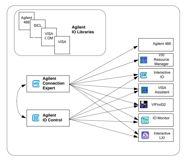
**Figure 2** Libraries and utilities that make up Agilent IO Libraries Suite. The Agilent Connection Expert and Agilent IO Control provide access to the other IO Libraries Suite utilities, as shown by the arrows.
