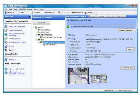
Figure 54 Agilent Connection Expert - USB Interface Selected
