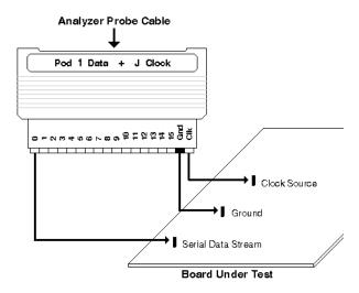
If multiple clock signals are required "to set up the state sampling clock" (in the online help), multiple logic analyzer pods are required. Each pod has one clock channel available.
