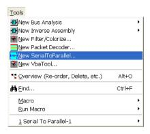
Or, in the Overview window, from a logic analyzer module's drop-down menu, choose **New Tool>SerialToParallel**.
