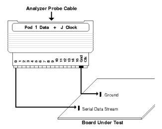
The pictures above show the flying-lead probe set, but there are many other options for probing a device under test. For more information on the available probing options, see "Probing the Device Under Test" (in the online help).
