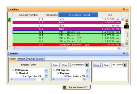
Both the Packet Decoder tool and the Packet Viewer window work with multiple protocols, specified by XML-format protocol description files.
