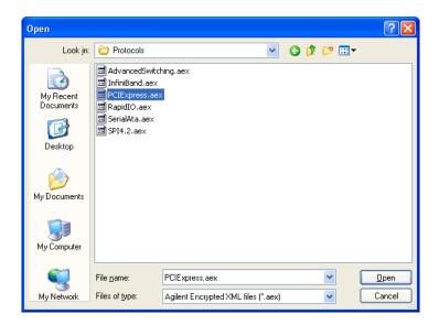
Protocol description files have the .aex (Agilent Encrypted XML) file extension.
