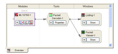
There is also a Packet Viewer window that displays decoded packet information.
