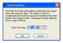
The clock out delay setting lets you position the output clock with respect to the data. The zero setting is uncalibrated and should be measured to determine the initial position with respect to the data. You can delay the clock in 500 ps increments.
