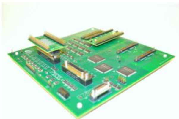
Cryogenic multi-layer circuit board designed in the CfD and populated in CEMA. Components on this board will be exposed to temperatures as low as 40 K, nanoTorr pressure, and high energy particle radiation.
