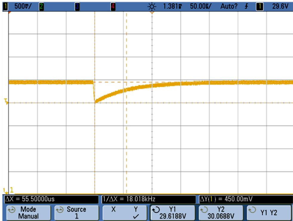
Figure 29 – Passive Quench Screen Capture with Cursor Measurements
