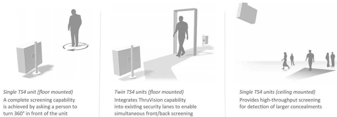
Figure 1.7.: Example ThruVision system concepts for security screening. ThruVision systems are active operating in the 0.25 THz wavelength region. Reprinted from [7]
