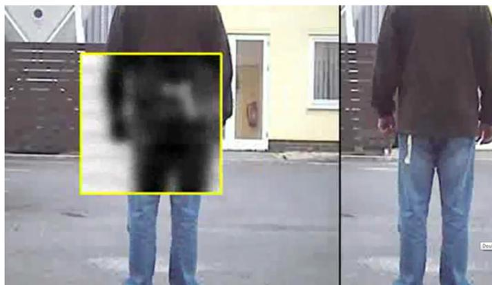
Figure 1.8.: Example image from ThruVision system. The inset on the left shows an overlaid THz image and the presence of a handgun under the subject's clothing. Reprinted from [7]
