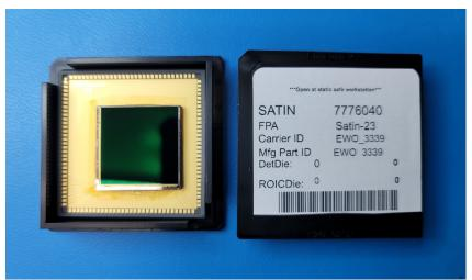
Figure 1. The image shows the VIRGO-V23 detector on the left and the container lid on the right.
