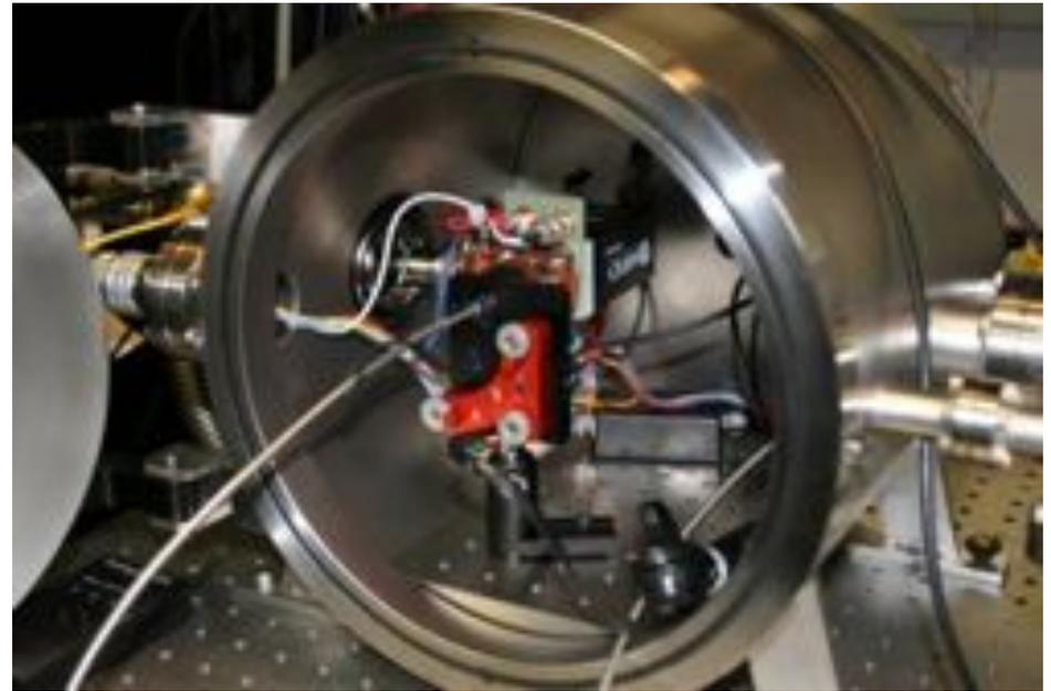
InGaAs or InGaAsP APD low temperature test chamber
