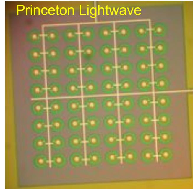
Packaged 32x32 InGaAs APD array on readout IC, with microlens array, on TE cooler inside package
