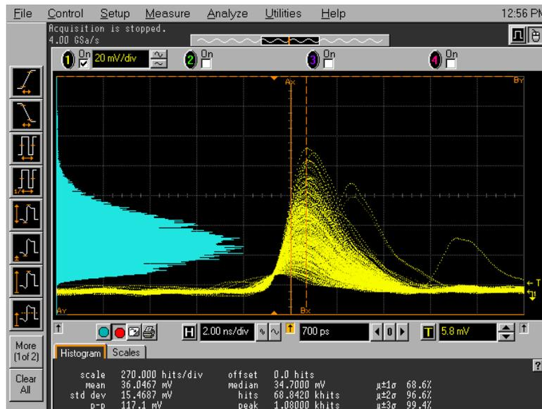
The excess noise factor may be obtained from pulse amplitude fluctuation under single photon detection, as,
