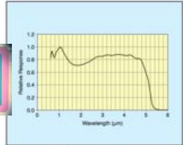
Figure 2: Relative spectral response of 5.1  $\mu\text{m}$  cutoff HgCdTe HDVTP at 80 K
