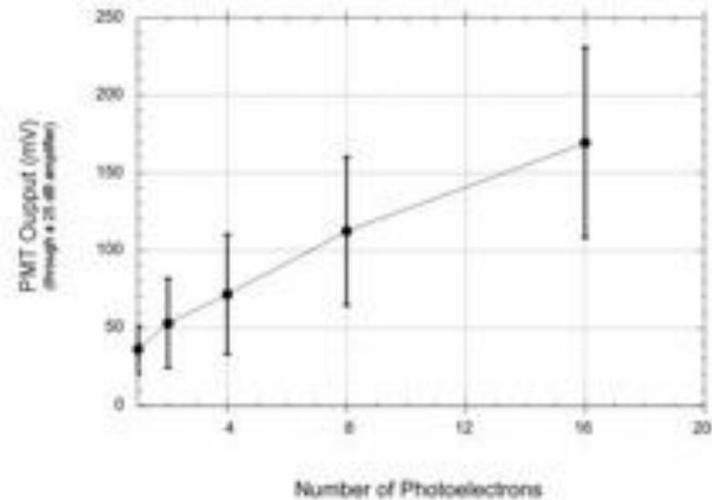
The excess noise factor is still too large to resolve the number of photons in the pulse (the error bars too large and overlaps for up to 16 detected photons, or 94 incident photons)
