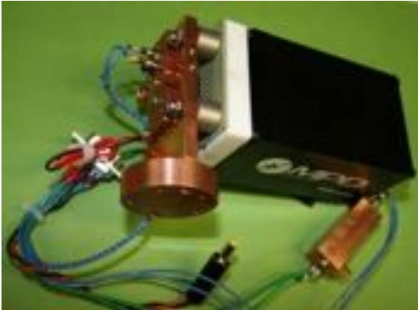
InGaAs or InGaAsP APD active quench circuit and cold finger mount
