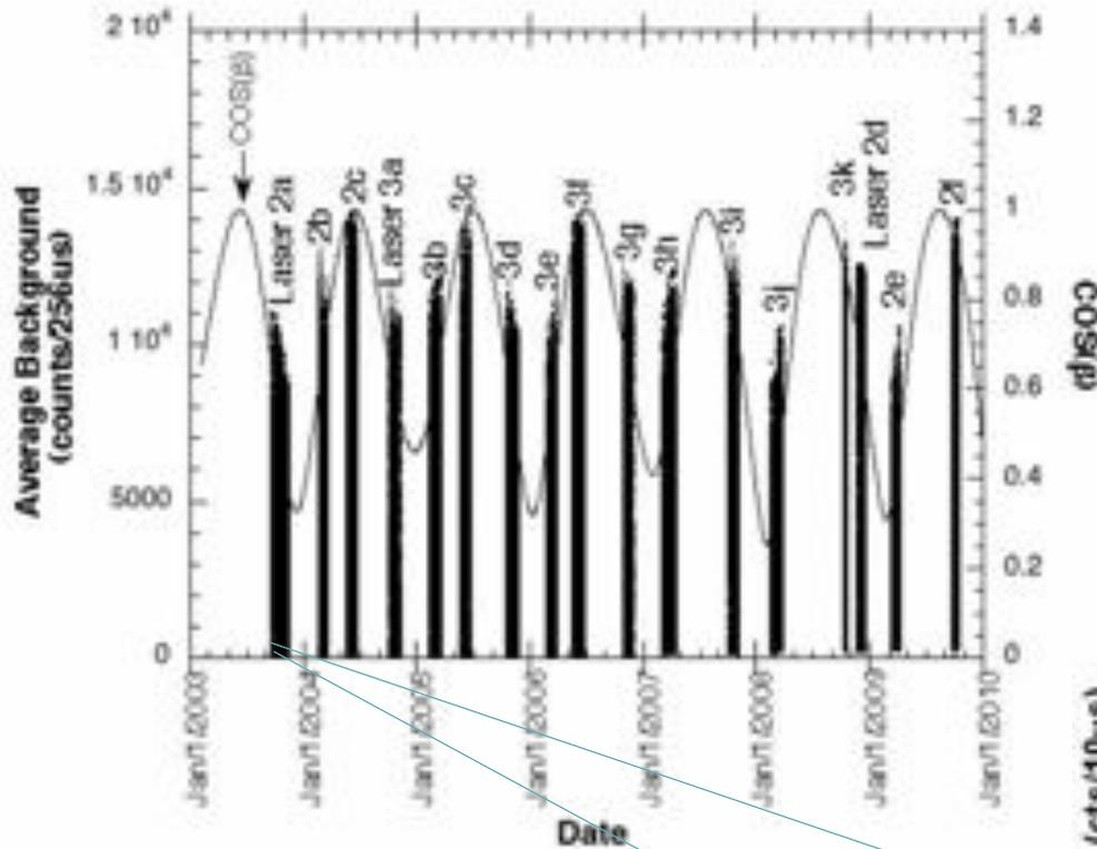
Daytime maximum count rate corresponded to the solar energy intensity within the field of view
