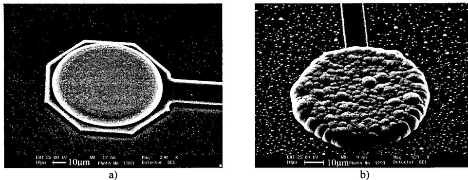
Figure 4. SEM micrographs of electroless Ni bumps a) 225µm pitch on wafer A, and b) 150µm pitch on wafer B
