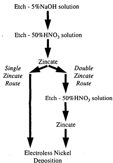
Figure 1: Process route for electroless Ni bumping of Al bondpads.
