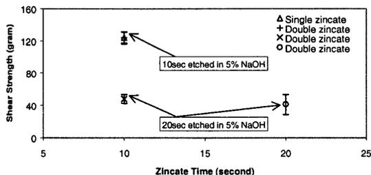
Figure 7. Shear test for 150µm pitch pads on wafer B
