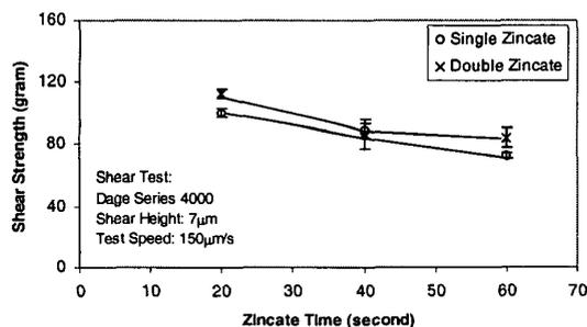
Figure 6. Shear test results for 225µm pitch bondpads on Wafer A
