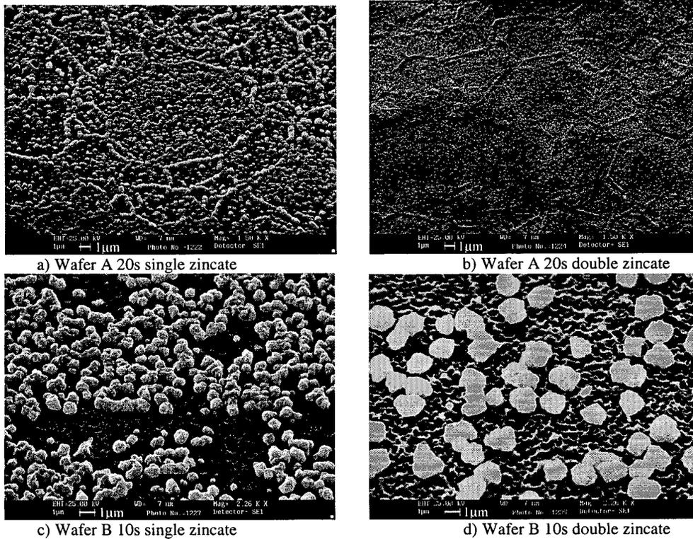
Figure 3. Zincate film characteristic after single and double zincate treatment
