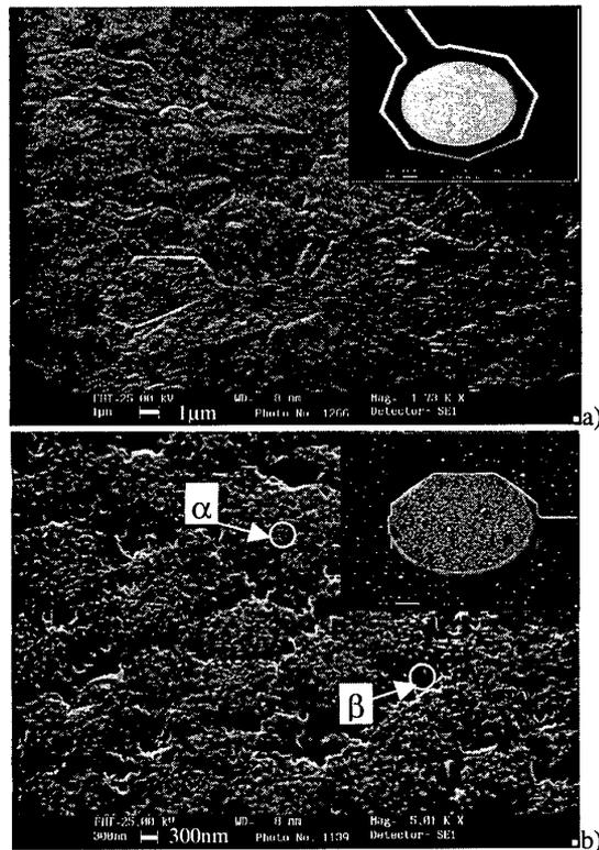
Figure 2. SEM micrographs of bond pads from a) wafer A, and b) wafer B.
