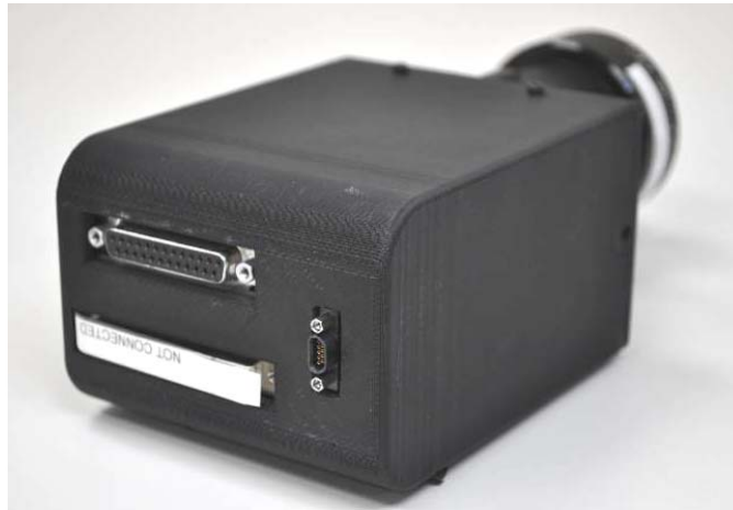
Figure 7: DRS U6000 Infrared Camera DB-25 Output Port and Power/RS-232 Connector
