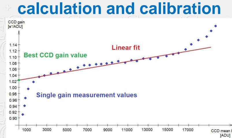
The CCD gain is calculated at different illumination levels using the statistical method and plotted as given. Then a fit is done from values above 1000 and below 15000 ADU and the intersection with the y-axis gives the best CCD gain value.
