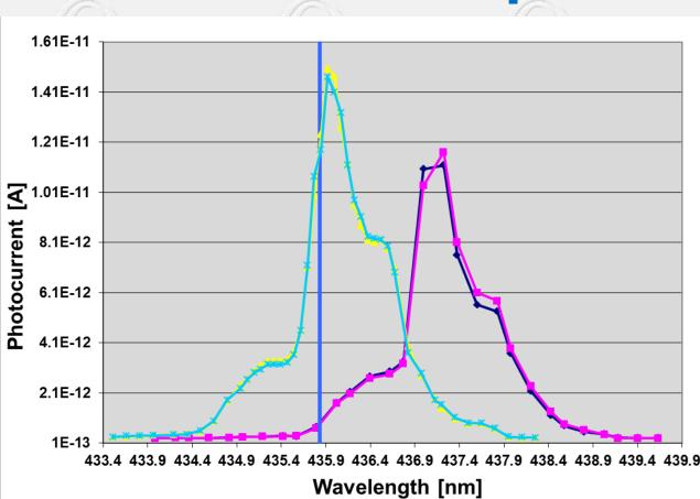
Calibration at 435.8 nm (blue vertical line): The pink-darkblue lines show measurements before calibration and the turqouis-yellow lines after the calibration. The acurracy of calibration is 0.086 nm (far better than needed!)
