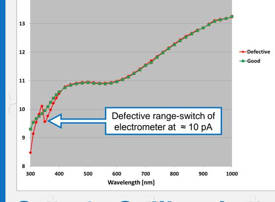
Measurement curve of defective (red) and correct calibrated (green) electrometer
