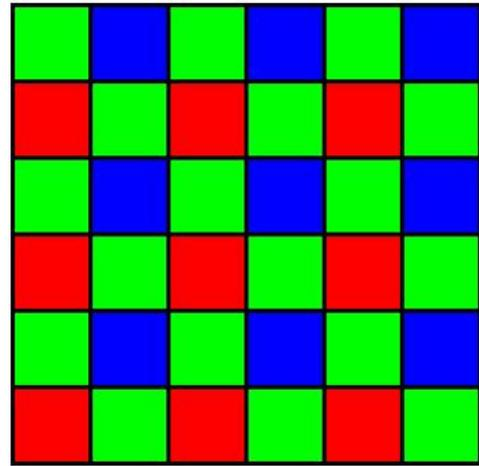
Fig. 2. Bayer Pattern color filter array applied to the camera sensor
