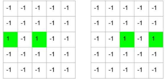
Fig. 4. Design of the two horizontal kernels used to identify cosmic ray damage, similar vertical and diagonal iterations are also used
