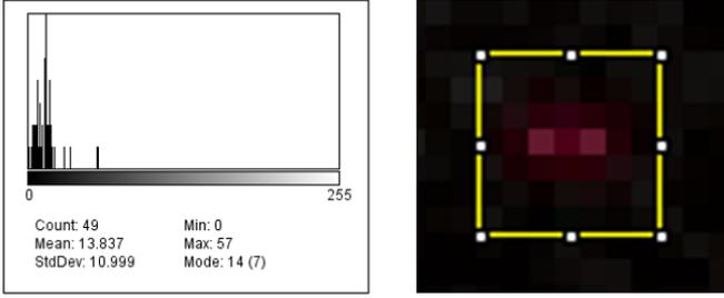
Fig. 3. Histogram of cosmic ray damage and background where the damage corresponds to the outliers of the distribution
