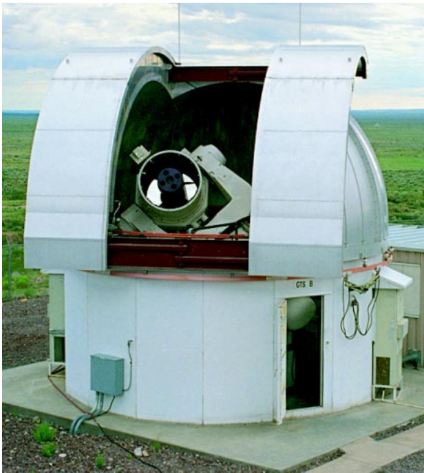
FIGURE 2. One of two one-meter Ground-Based Electro-Optical Deep-Space Surveillance (GEODSS) search telescopes at the Lincoln Laboratory Experimental Test System (ETS) at White Sands Missile Range, New Mexico. This telescope, which previously was used for space surveillance, is now a component of the Lincoln Near-Earth Asteroid Research (LINEAR) asteroid search program.
