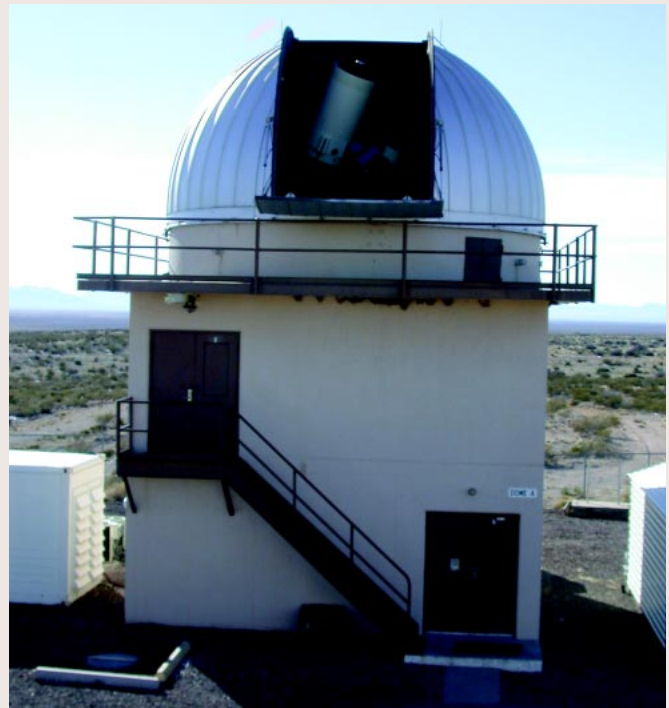
FIGURE B. The LINEAR 3 telescope and its dome at the Lincoln Laboratory–operated Experimental Test System in New Mexico. It is a Cassegrain telescope with a thirty-inch aperture and a 0.5 square-degree field of view. It can routinely detect objects with a visual magnitude of 19.0 with forty seconds of integration. (Photographs courtesy of Peter Trujillo.)
