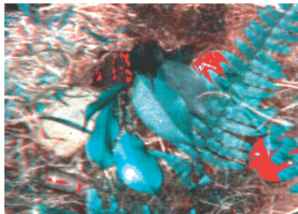
FIGURE 8. Detections, in red, of the plastic and metal targets. Fusion of the spectral-reflectance, polarization, and fluorescence data allows us to detect the metal shell casing (bottom left), which we could not detect with active hyperspectral data alone.
