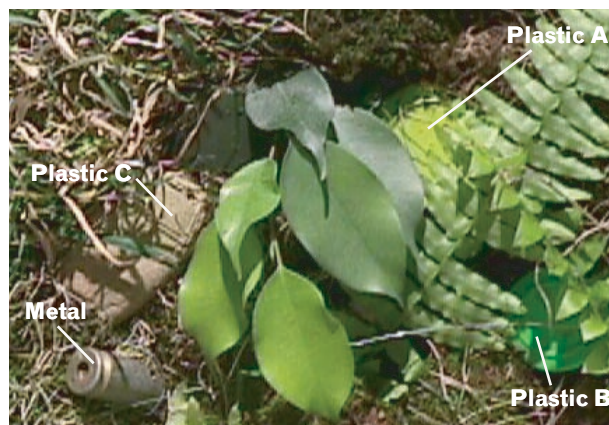
FIGURE 5. Digital-camera photo of the target scene, containing soil, vegetation, rocks, sticks, three different types of plastic, and a metal shell casing.
