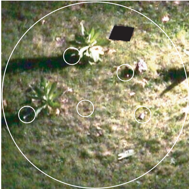
FIGURE 11. Photograph of the imaged scene comprising five inert land mines amidst clutter of rocks, sticks, and vegetation. White circles indicate target positions and the black square indicates the position of the calibration panel.
