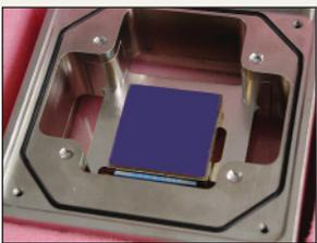
Figure 1: The Rockwell H2RG Sensor-Chip Array (SCA).
