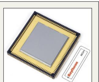
Figure 2: Raytheon multiplexer for the mid-infrared detector.
