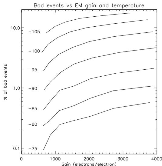
Fig. 9.— Fraction of bad events as a function of the EM gain and temperature (in  $^{\circ}\text{C}$ ), as measured with CCCP/CCD97. The bad event rate shown in this figure is not compensated from the natural rate at which two adjacent events can occur.
