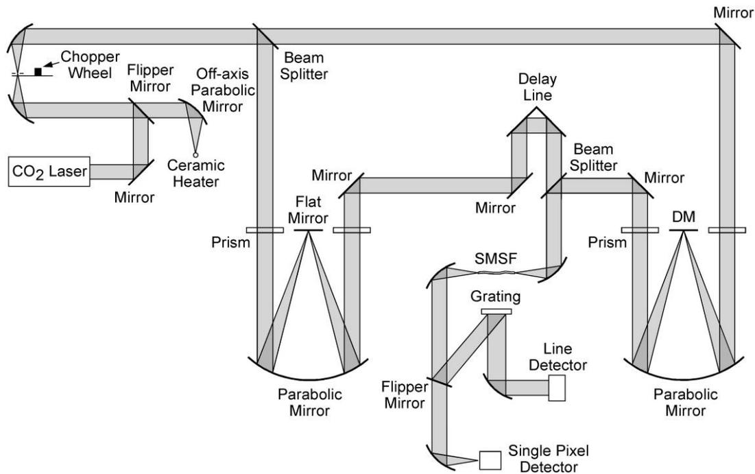
FIG. 2.—Schematic of the adaptive nulling lab experiment.
