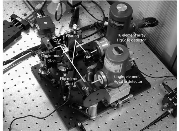
FIG. 4.—Photo of the detector system. A flip mirror can be used to select between a single-pixel detector used for null measurements and the spectrometer used to initialize the phase and intensity corrections. See the electronic edition of the *PASP* for a color version of this figure.
