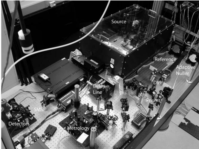
FIG. 3.—Overview of the Adaptive Nuller testbed. The interferometer uses a Mach-Zehnder arrangement with a reference arm and an arm with an adaptive corrector. The light is then recombined and sent to through a mid-infrared single-mode fiber to the detectors, shown on the *left*. Additional details of the testbed design are given by Peters et al. (2008). See the electronic edition of the *PASP* for a color version of this figure.
