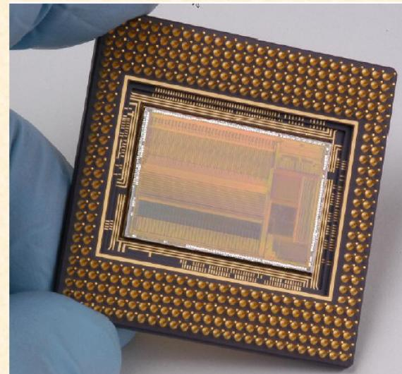
**Figure 2:** Image of the SIDECAR. All signal conditioning, clock/bias generation and digitization hardware is self-contained in this small chip.
