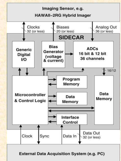
**Figure 5:** Block diagram of the SIDECAR
