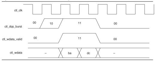
Figure 5–16 shows a full-rate write.
