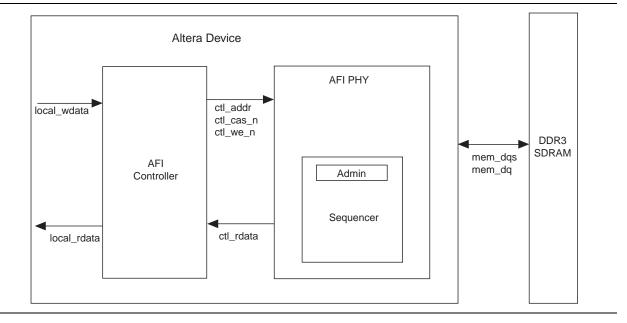
For half-rate designs, the address and command signals in the ALTMEMPHY megafunction are asserted for one mem\_clk cycle (1T addressing), such that there are two input bits per address and command pin in half-rate designs. If you require a more conservative 2T addressing, drive both input bits (of the address and command signal) identically in half-rate designs.
