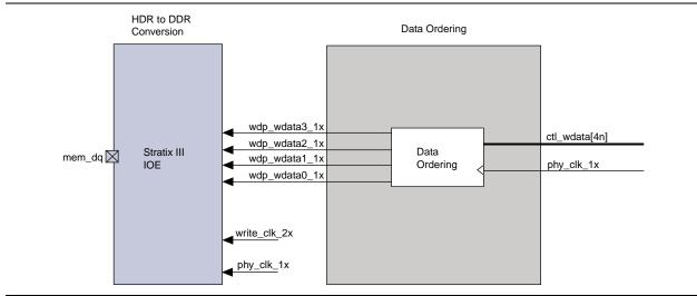
All of the write datapath registers in the Stratix IV and Stratix III devices are clocked by the half-rate clock, phy\_clk\_1x.
