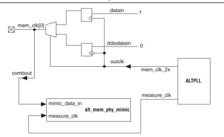
Figure 5–3. Mimic Path in Arria GX, Arria II GX, Cyclone III, Stratix II, and Stratix II GX Devices
