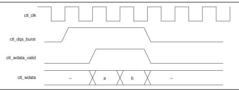
After calibration completes, the sequencer sends the write latency in number of clock cycles to the controller.
