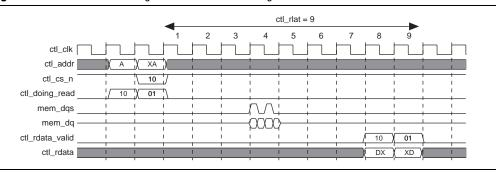
Figure 5-24. Second Read Alignment—Half-Rate Design
