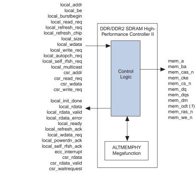
Figure 7–1. DDR and DDR2 SDRAM HPC II Block Diagram
