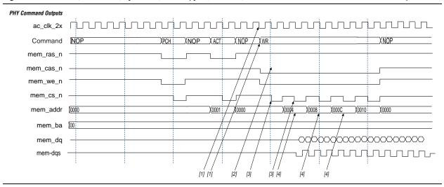
Figure 5-4. Arria GX, Arria II GX, Cyclone II, HardCopy III, Stratix II, and Stratix II GX Address and Command Datapath
