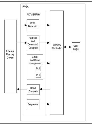
Figure 5-1. ALTMEMPHY Megafunction Interfacing with the Controller and the External Memory
