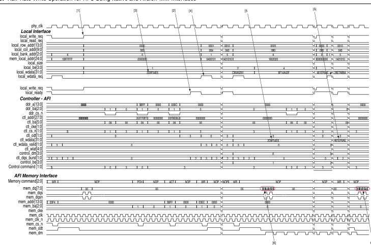
Figure 9–6. Half-Rate Write Operation for HPC Using Native and Avalon-MM Interfaces
