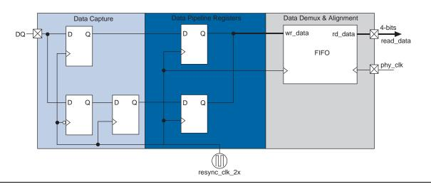
The full-rate read datapath for Cyclone III devices is similar to the half-rate Cyclone III implementation, except that the data is read out of the FIFO buffer with a full-rate clock instead of a half-rate clock.
