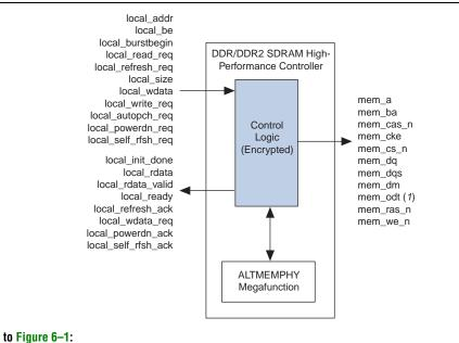
Figure 6–1. DDR and DDR2 SDRAM HPC Block Diagram
