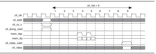
Figure 5–23. Address and Command and Read-Path Timing—Full-Rate Design
