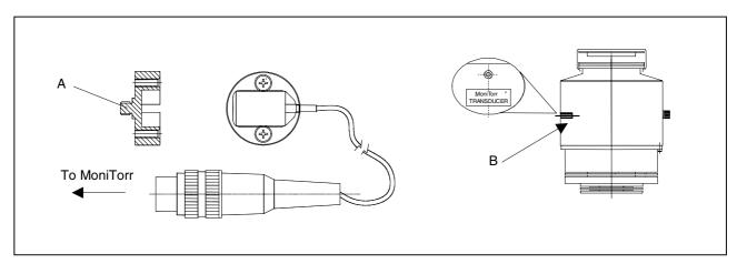
Accelerometer Support for ICE and 2000 HT Series Turbopumps
