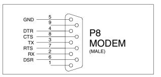
RS232 Serial Connector for the Modem
