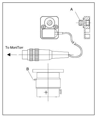
Accelerometer Support for HT Series Turbopumps
