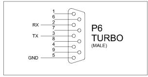
RS 232 Data Exchange Serial Port Connections
