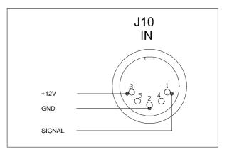
Connector J10 (Accelerometer)
