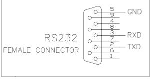
RS 232 Data Exchange Serial Port Connections
