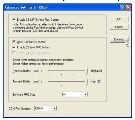
5. Check/un-check the "Enable CTS/RTS Auto Flow Control" checkbox to enable/ disable the hardware auto flow control feature.
