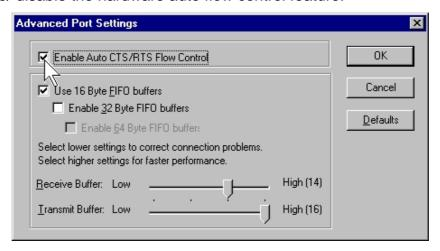
6. Check/Un-check the "Use 16 Byte FIFO buffers" or "Use 32 Byte FIFO buffers" checkbox to enable / disable the hardware FIFO buffering feature or you can select the size of FIFO if "Use FIFO buffers control" is enabled.
