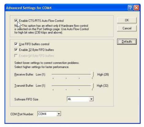
Check/Un-check the "Use FIFO buffers control" checkbox to enable / disable the hardware FIFO buffering feature or you can select the size of FIFO if "Use FIFO buffers control" is enabled.
