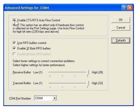
6. Check/Un-check the "**Use FIFO buffers control**" checkbox to enable / disable the hardware FIFO buffering feature or you can select the size of FIFO if "Use FIFO buffers control" is enabled.
