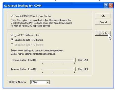
5. Check/un-check the "Enable CTS/RTS Auto Flow Control" checkbox to enable/ disable the hardware auto flow control feature.
