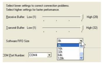
This FIFO is used to buffer data on the receive path. The size of the FIFO can be configured in the advanced property page of the driver. It allows setting between 128byte to 128 kilo byte. The setting of the software size can be chosen individually for each port.
