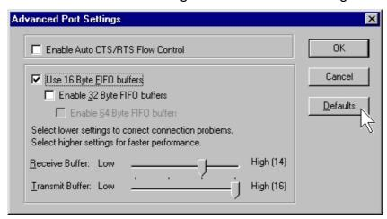
5. Check/un-check the "Enable CTS/RTS Auto Flow Control" checkbox to enable/ disable the hardware auto flow control feature.
