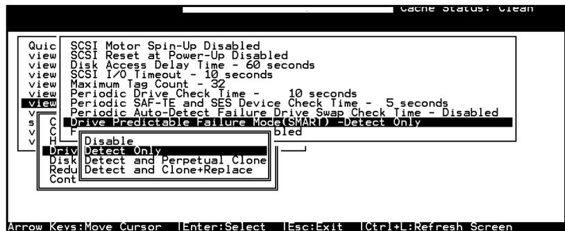
3b. Whenever a drive predicts symptoms of predictable drive failure, controller will issue an error message.
