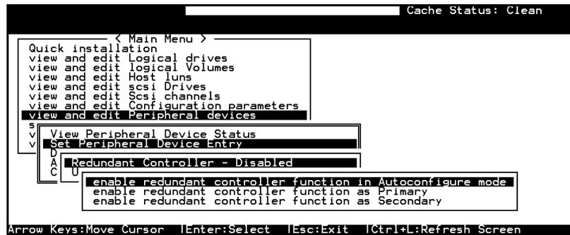
When the new controller is connected, the existing controller will automatically start initializing the replacement controller (IFT-3102U2G and above). If the existing controller does not initialize the replacement controller, execute the "Deassert Reset on Failed Controller" function.
