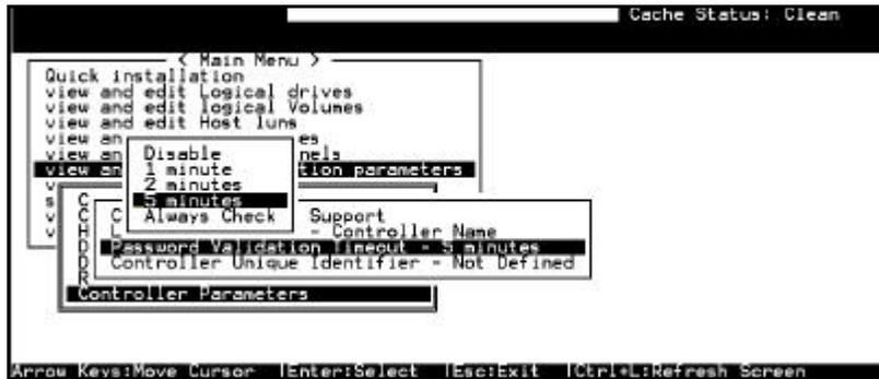
Choose “View and Edit Configuration parameters,” “Controller Parameters,” then press [ENTER]. Select “Password Validation Timeout,” and press [ENTER]. Choose to enable a validation timeout from one minute to always check. The always check timeout will disable any configuration change without entering the correct password.
