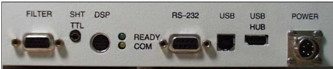
Figure 10. Cable Connections (Back Panel)
