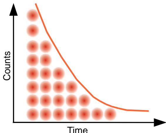
Fig. 2: Fluorescence lifetime histogram: exponential decay
