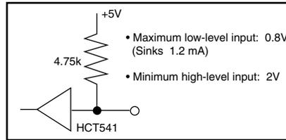
**Output #1 (Signal 10) and Output #2 (Signal 8)**
