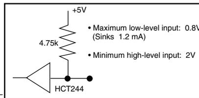
**Trigger Inputs #1 - #3 (Signals 20 - 22)**
