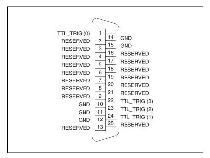
Figure A-2. 25-Pin D-SUB Trigger Connector
