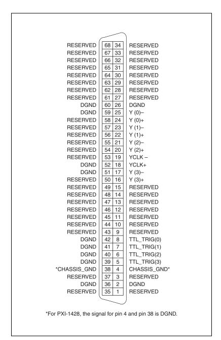
Figure 3-3. NI 1428 68-Pin VHDCI Connector Pin Assignments
