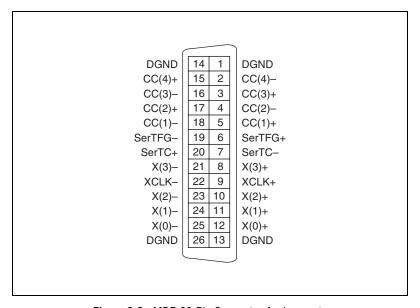
Figure 3-2. MDR 26-Pin Connector Assignments
