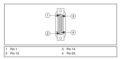
Figure 4. 25-Pin D-SUB Connector (Cable)
