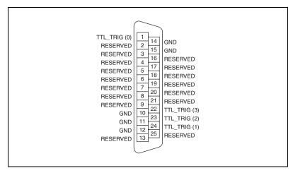
Figure 5. 25-Pin D-SUB Trigger Connector Pinout (Cable)
