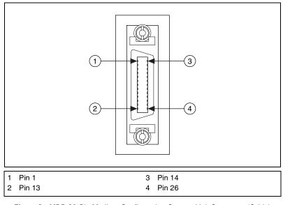
Figure 3. MDR 26-Pin Medium Configuration Camera Link Connector (Cable)
