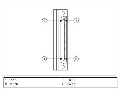
Figure 2. 68-Pin VHDCI Connector (Cable)
