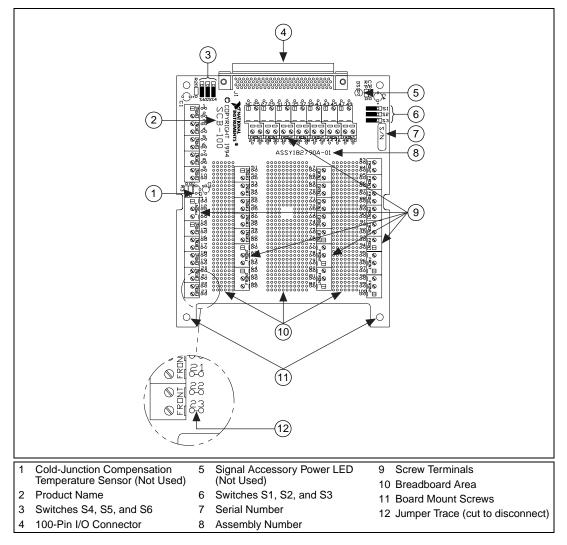
Figure 3. IMAQ SCB-100 Terminal Block Parts Locator Diagram
