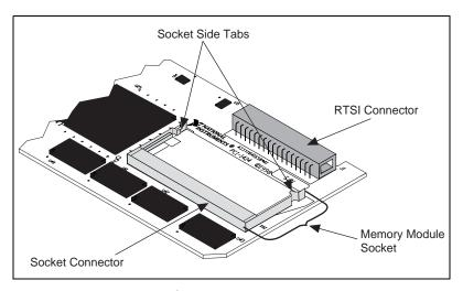
Figure 1. PCI-1424 Memory Module Location
