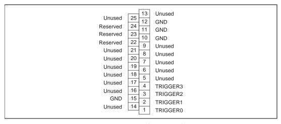
Figure 2. D100 Cable Trigger Connector Pin Assignments
