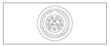
Figure 3. Hirose Connector (Cable)
