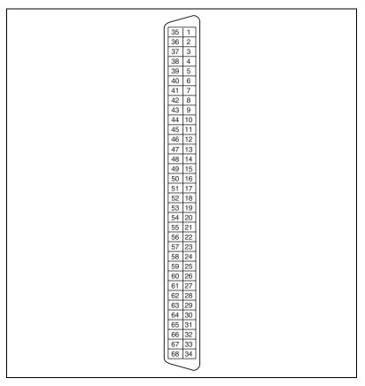
Figure 2. 68-Pin VHDCI Connector (Cable)
