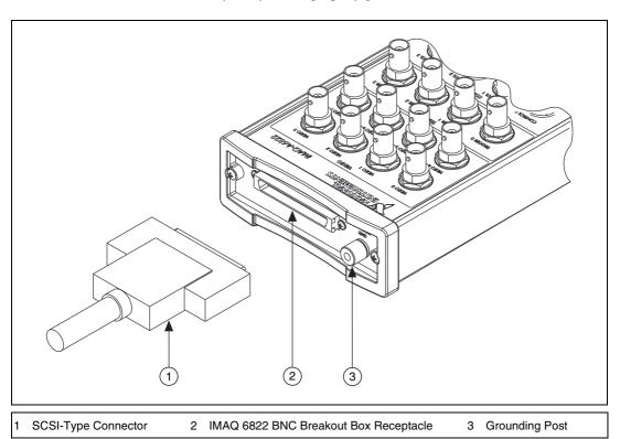
Figure 1. IMAQ 6822 BNC Breakout Box and Cable
