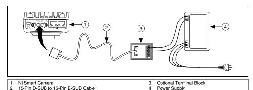
Figure 2. Connecting the NI Smart Camera to a Third-Party Power Supply
