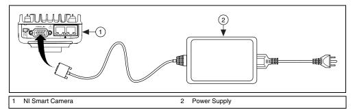
Figure 1. Connecting the NI Smart Camera to the NI Desktop Power Supply
