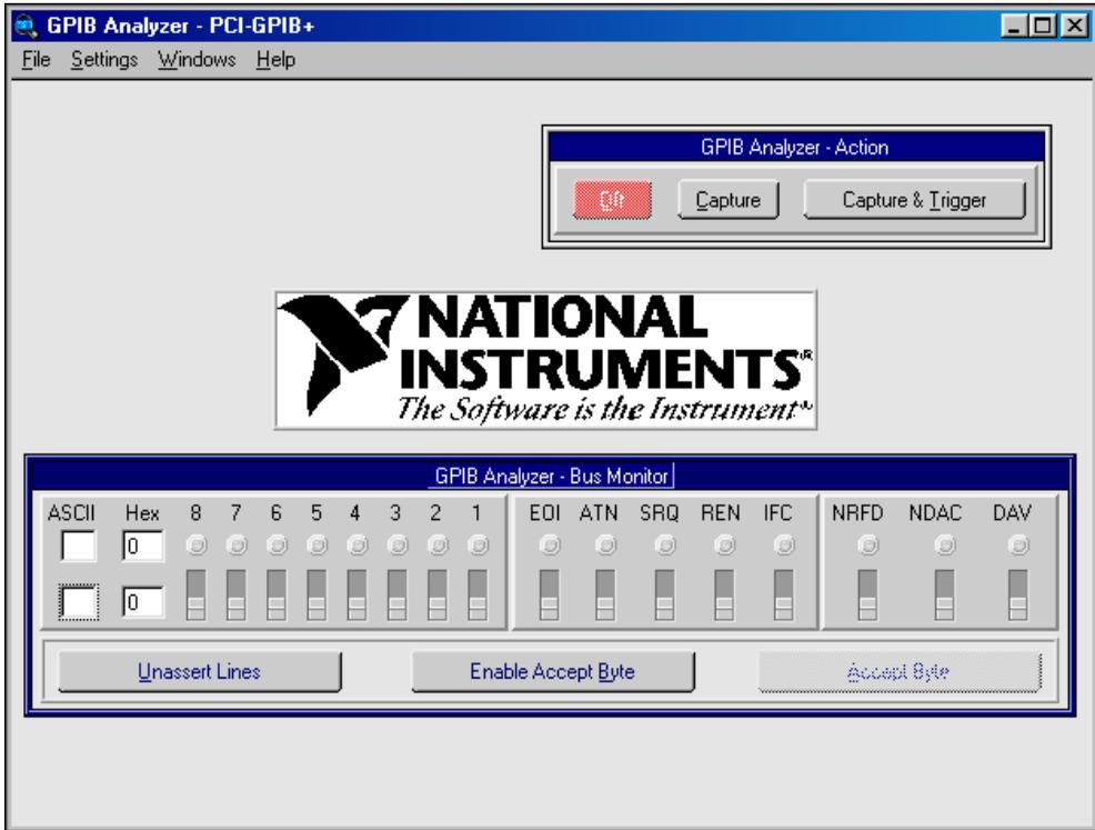
Figure 2-1. Main Window of the GPIB Analyzer
