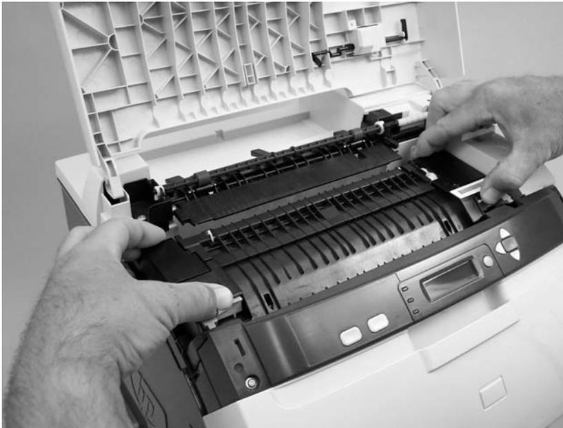
**Figure 5-12** Remove the upper cover (2 of 5)
