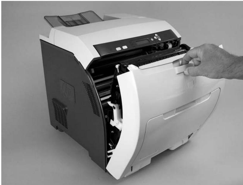
3. Rotate the transfer unit up and away from the front cover.
