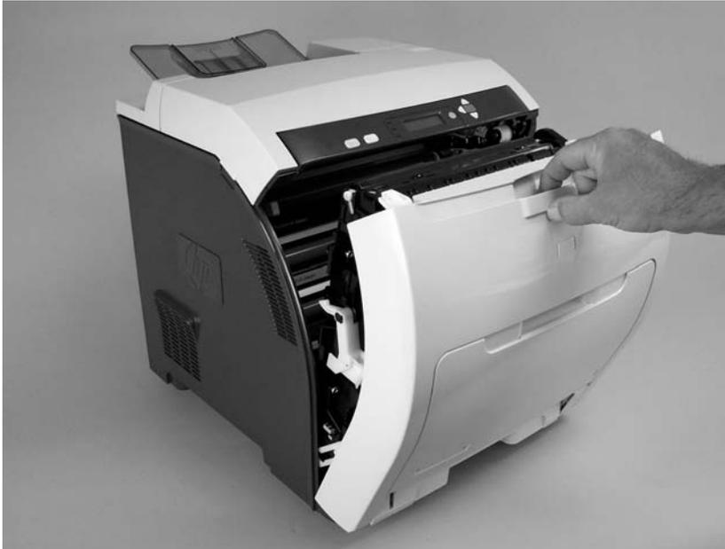
**Figure 5-2** Remove the print cartridges (1 of 2)
