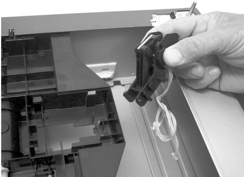
**Figure 5-127** Remove the media sensor (500-sheet feeder) (4 of 4)
