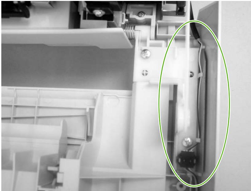
4. Disconnect one connector (callout 4) and remove the fan.
