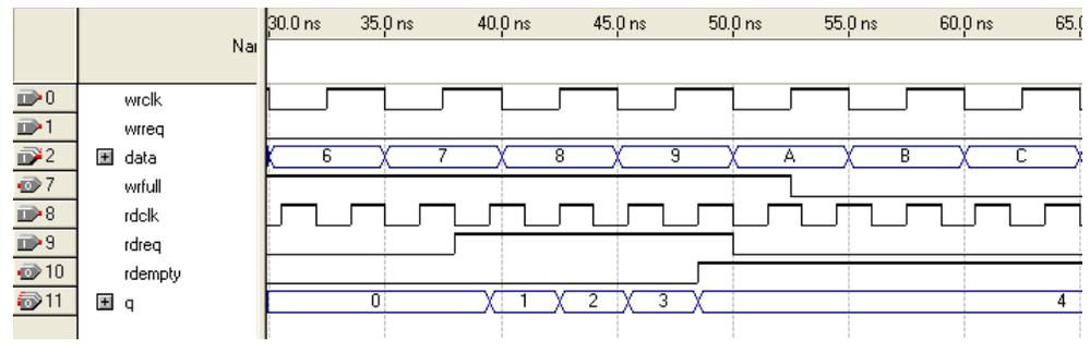
The required functional timing for the DCFIFO as described previously is also applied to the SCFIFO. The difference between the two modes is that for the SCFIFO, the wrreq signal is with respect to full flag and the rdreq signal is with respect to the empty flag.
