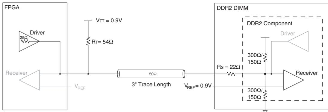
[Figure 5](#) shows a HyperLynx simulation and board measurements of a signal seen at the memory of a double parallel termination using ODT 150 Ω with a memory-side series resistor transmission line when the FPGA is writing to the memory with a 25-Ω OCT drive strength setting.
