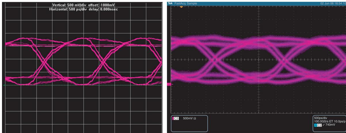
Table 7 summarizes the comparison of the signal at the memory of a dual-DIMM memory interface with one slot and with both slots populated using a double parallel termination using an ODT setting of  $75\ \Omega$  with a memory-side series resistor with a  $25\text{-}\Omega$  OCT strength setting on the FPGA.
