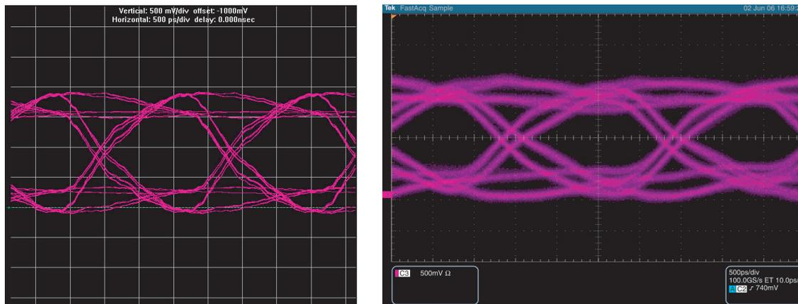
Table 13 summarizes the comparison between the simulation and board measurements of the signal seen at the memory in slot 1 of a dual-DIMM memory interface with both slots populated using a double parallel termination using a different ODT setting on Slot 2 with a memory-side series resistor with a 25-Ω OCT strength setting on the FPGA.
