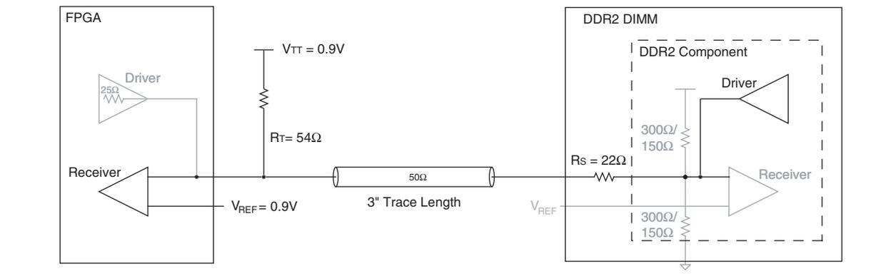
Figure 7 shows the simulation and measurements result of the signal seen at the FPGA of a single parallel termination using an external parallel resistor on the FPGA side with a memory-side series resistor with full drive strength setting on the memory.
