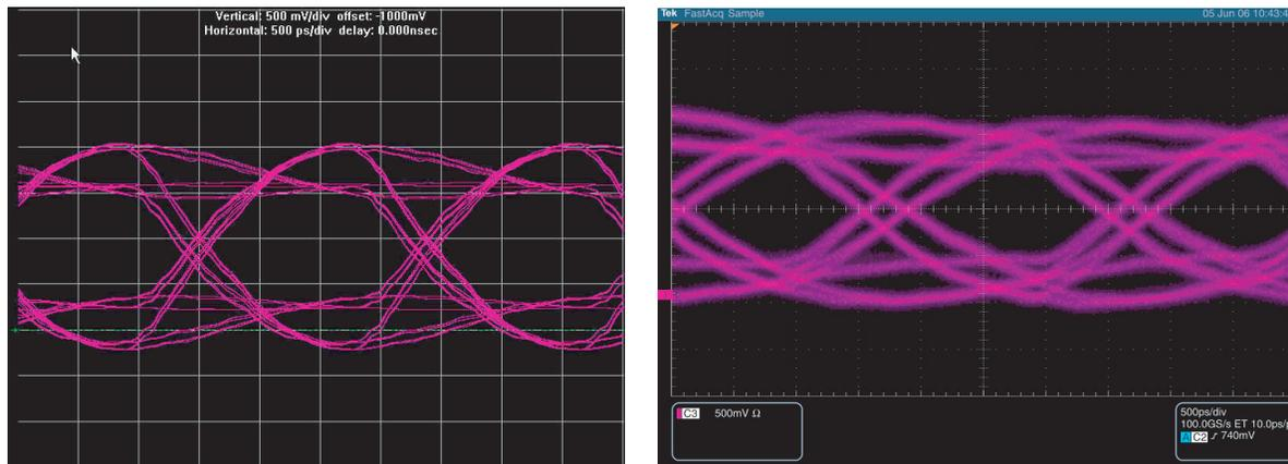
Table 14 summarizes the comparison between the simulation and board measurements of the signal seen at the memory of a dual-DIMM memory interface with both slots populated using a double parallel termination using a different ODT setting on Slot 1 with a memory-side series resistor with a 25-Ω OCT strength setting on the FPGA.
