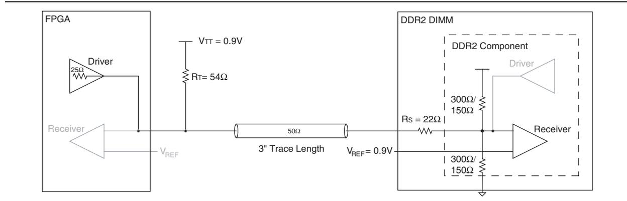
Figure 9 shows the simulation and measurements result of the signal seen at the memory of a double parallel termination using an ODT setting of 150 Ω with a memory-side series resistor transmission line when the FPGA is writing to the memory with a 25-Ω OCT drive strength setting.
