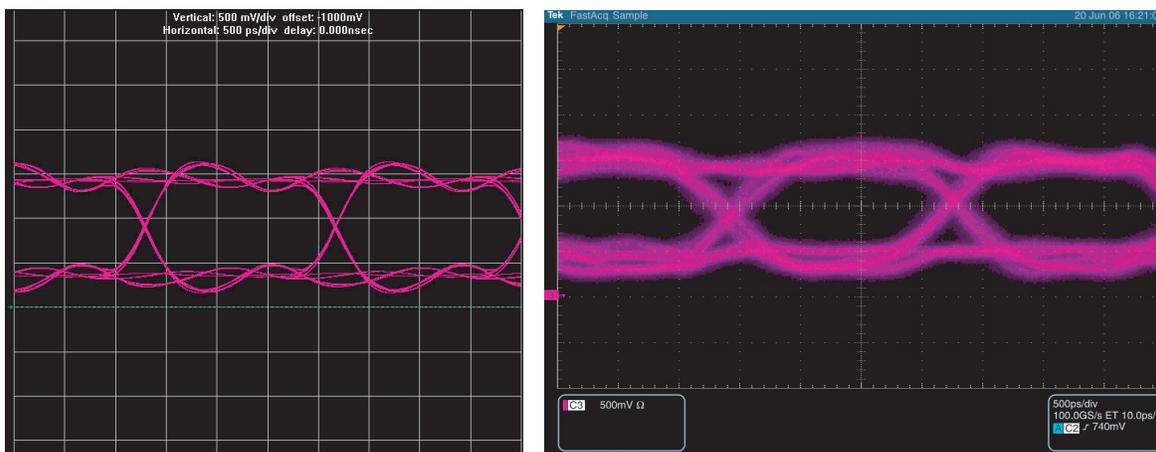
Table 11 summarizes the comparison between the simulation and board measurements of the signal seen at the DDR2 SDRAM of a dual-DIMM with slot 1 populated by a memory interface using a different ODT setting.
