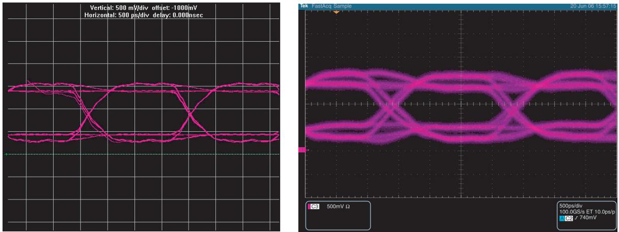
Table 12 summarizes the comparison of the signal at the memory of a dual-DIMM memory interface with either slot 1 or slot 2 populated using a double parallel termination using an ODT setting of  $75\ \Omega$  with a memory-side series resistor with a  $25\text{-}\Omega$  OCT strength setting on the FPGA.
