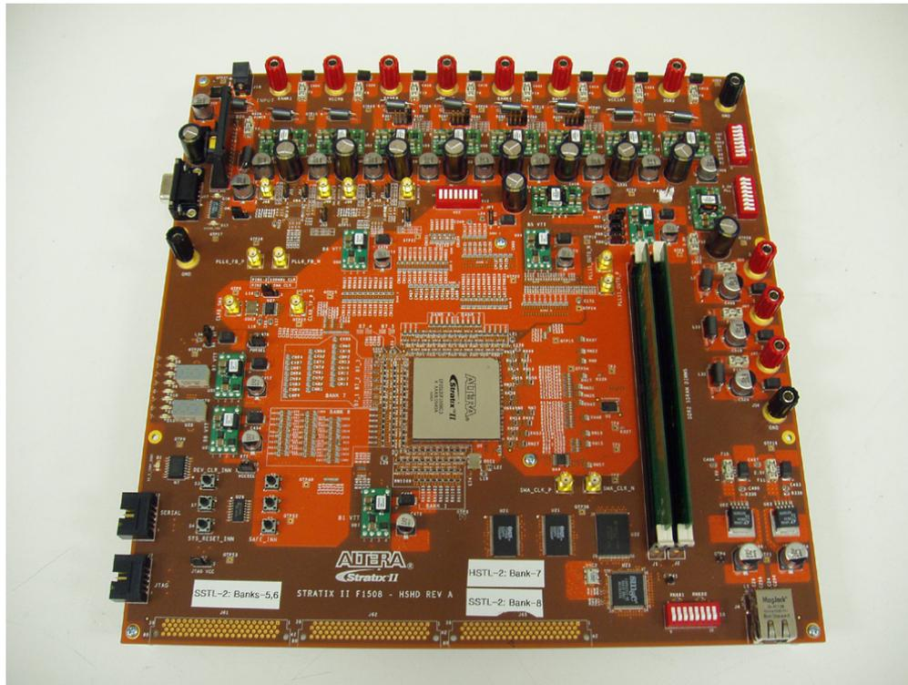
The Stratix II High-Speed Board uses a Stratix II 2S90F1508 device. For DQS, DQ, and DM signals, the board is designed without external parallel termination resistors near the DDR2 SDRAM DIMMs, to take advantage of the ODT feature of the DDR2 SDRAM components. Stratix II FPGA devices are not equipped with dynamic OCT, so external parallel termination resistors are used at the FPGA end of the line.
