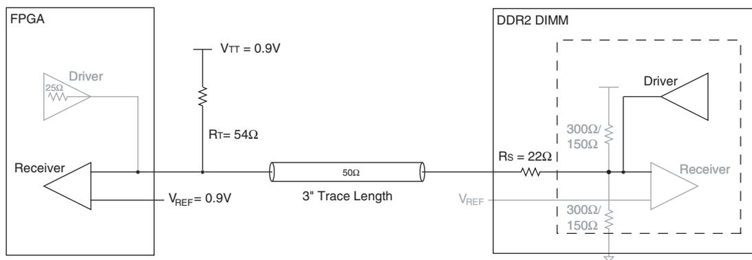
[Figure 11](#) shows the simulation and board measurements of the signal seen at the FPGA of a single parallel termination using an external parallel resistor on the FPGA side with a memory-side series resistor with full drive strength setting on the memory.
