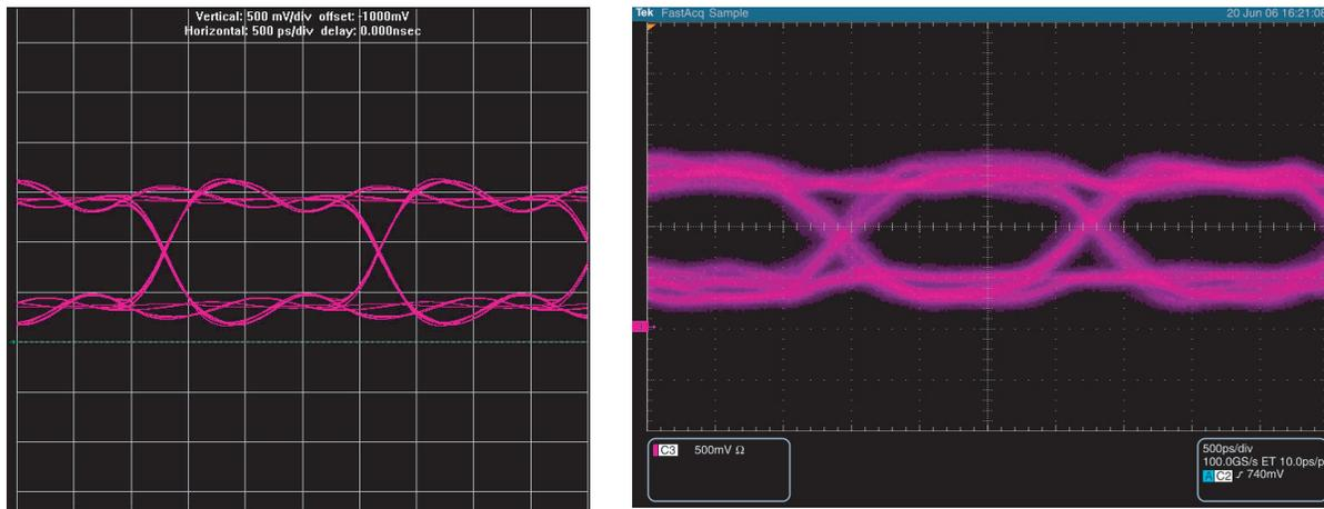
Table 6 summarizes the comparison between the simulation and board measurements of the signal seen at the FPGA of a dual-DIMM memory interface with either slot 1 or slot 2 populated using a single parallel termination using an external parallel resistor at the FPGA with a memory-side series resistor with full strength setting on the memory.
