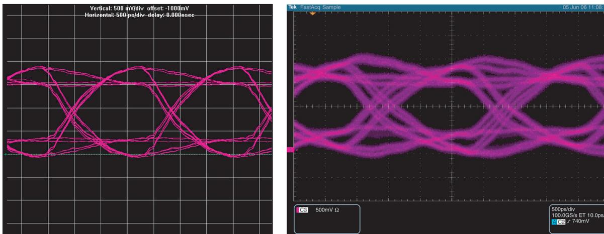
Table 8 summarizes the comparison of the signal at the memory of a dual-DIMM memory interface with slot 1 populated using a double parallel termination using an ODT setting of 75 Ω with a memory-side series resistor with a 25-Ω OCT strength setting on the FPGA.
