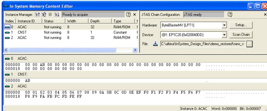
The Instance Manager displays all available run-time modifiable memories and constants in your FPGA device. The JTAG Chain Configuration section allows you to program your FPGA and select the Altera® device in the chain to update.
