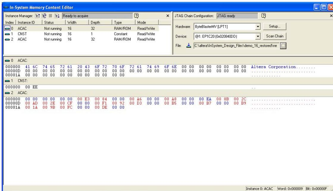
Unprintable ASCII characters are represented by a period (.). The color of the data changes as you perform reads and writes. Data displayed in black indicates the data in the Hex Editor was the same as the data read from the device. If the data in the Hex Editor changes color to red, the data previously shown in the Hex Editor was different from the data read from the device.
