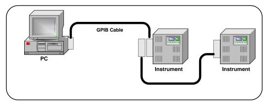
Figure 16 Typical GPIB System
