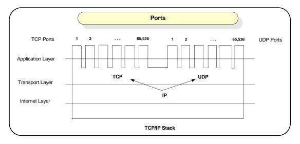
Figure 60 TCP/IP Protocol Stack
