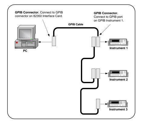
Figure 12 Connecting Three GPIB Instruments
