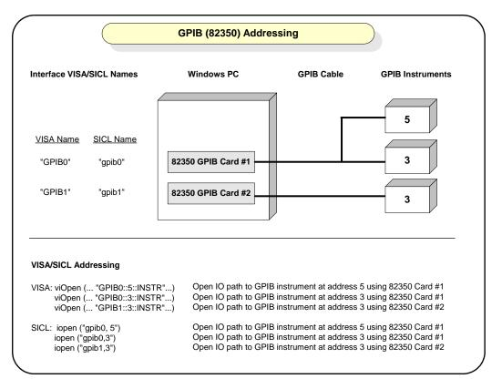
The GPIB interface system consists of a Windows PC with two 82350 GPIB cards connected to three GPIB instruments via GPIB cables. For this system, Connection Expert has been used to assign GPIB card #1 a VISA interface ID of "GPIB0" and a SICL interface ID of "gpib0".
