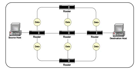
Figure 56 Example of Packet-Switched Network
