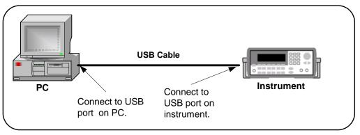
Figure 17 Typical USB Interface System
