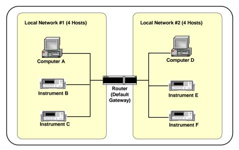
Figure 62 Two Networks (Subnets) Using a Router
