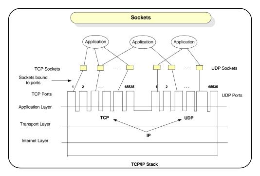
Figure 61 Typical Socket Architecture
