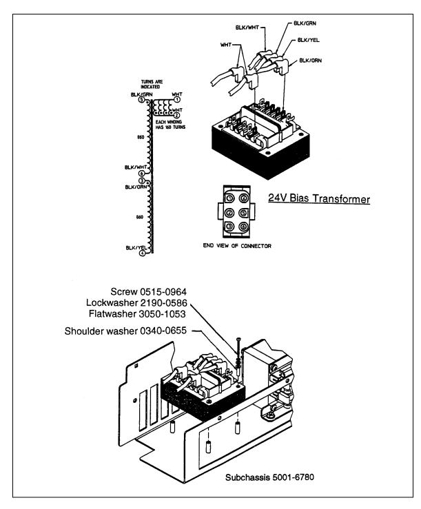
Figure 3-20. 24 Volt Fan Transformer
