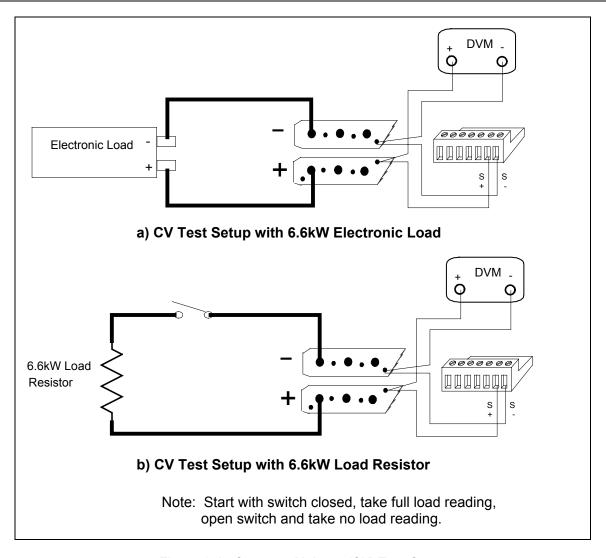
Figure 2-1. Constant Voltage (CV) Test Setup
