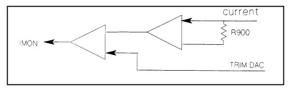
Figure 4-1. AC Calibration of IMON
