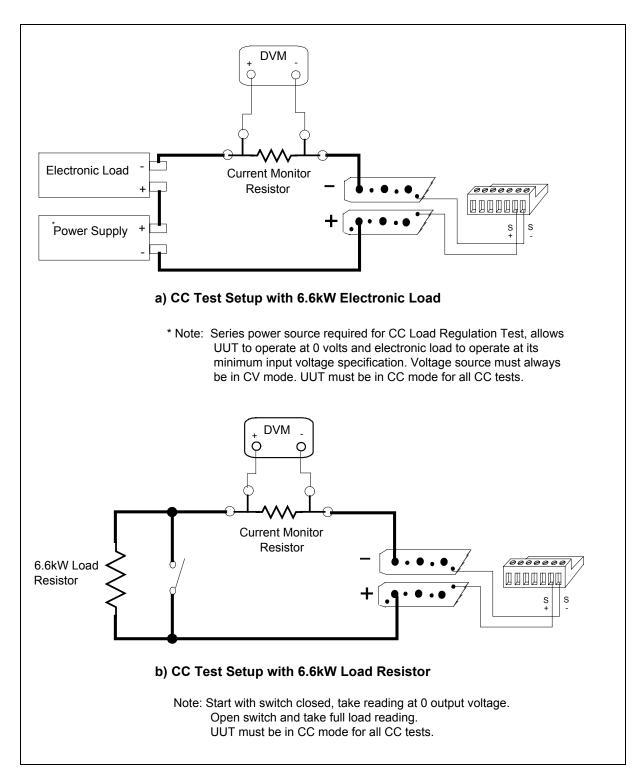
Figure 2-3. CC Load Effect Test Setup
