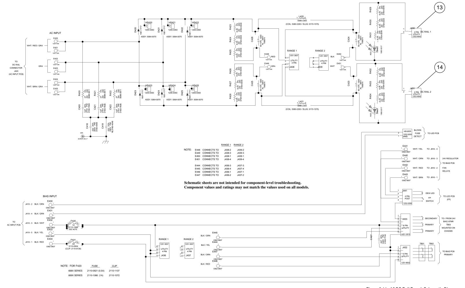
Figure 6-14. A5 DC Rail Board, Schematic Diagram
