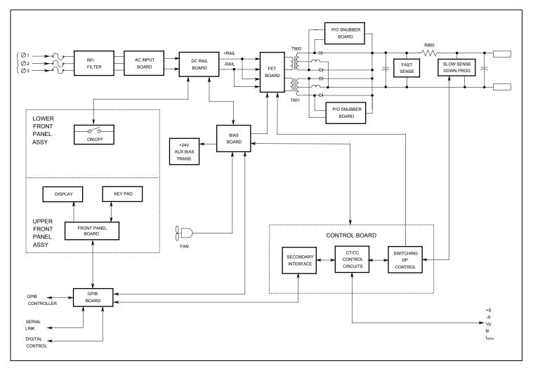
Figure 4-3. Agilent Series 669xA Power Supply, Block Diagram
