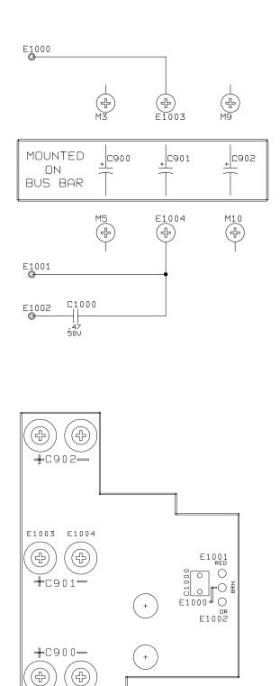
Figure 6-18. A7 Snubber Board, Component Location and Schematic Diagram
