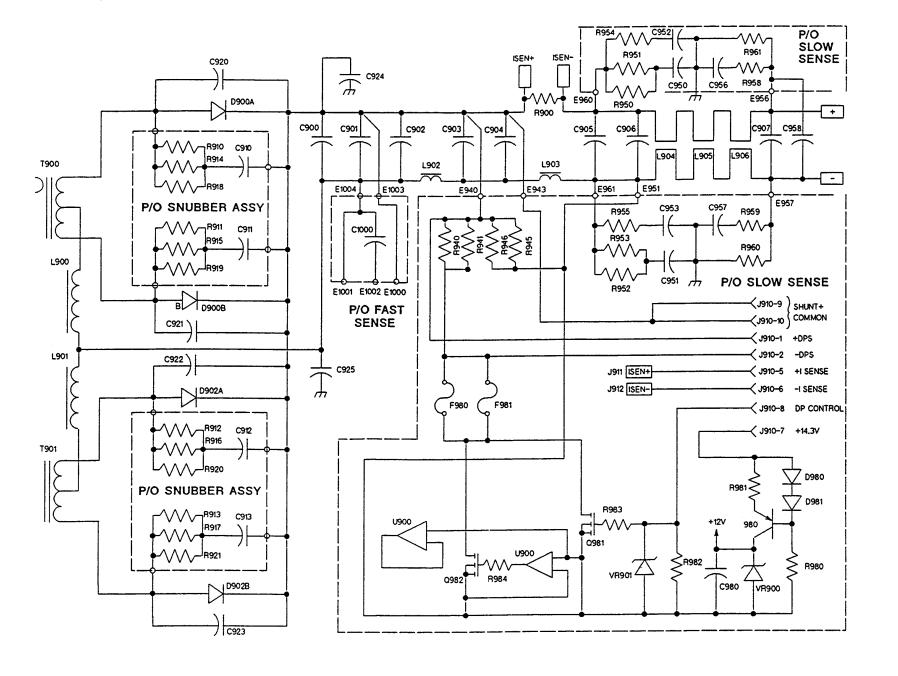
Figure 6-17. Power Mesh, Schematic Diagram, All Models
