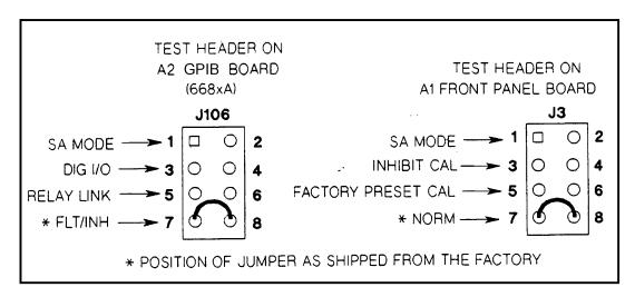
Figure 3-12. Test Header Jumper Positions
