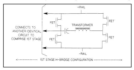
Figure 4-2. 1ST Stage of the FET H-Bridge Configuration
