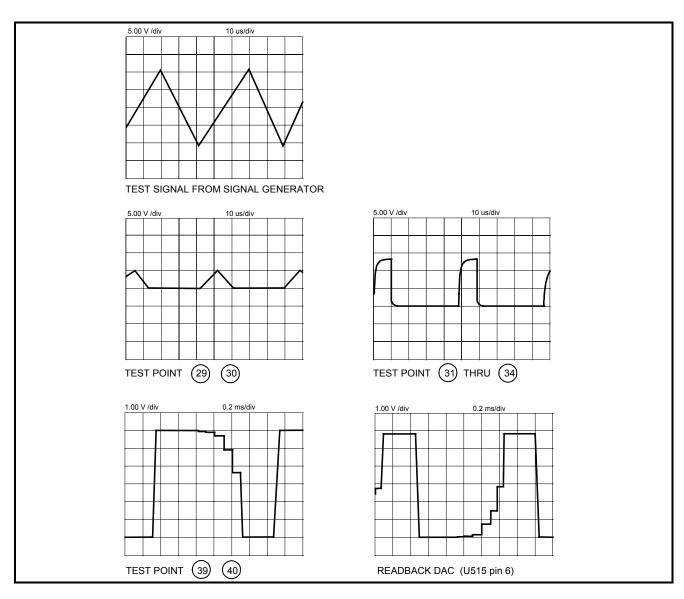
Figure 6-1. Test Point Waveforms for Table 6-3 (sheet 1 of 2)
