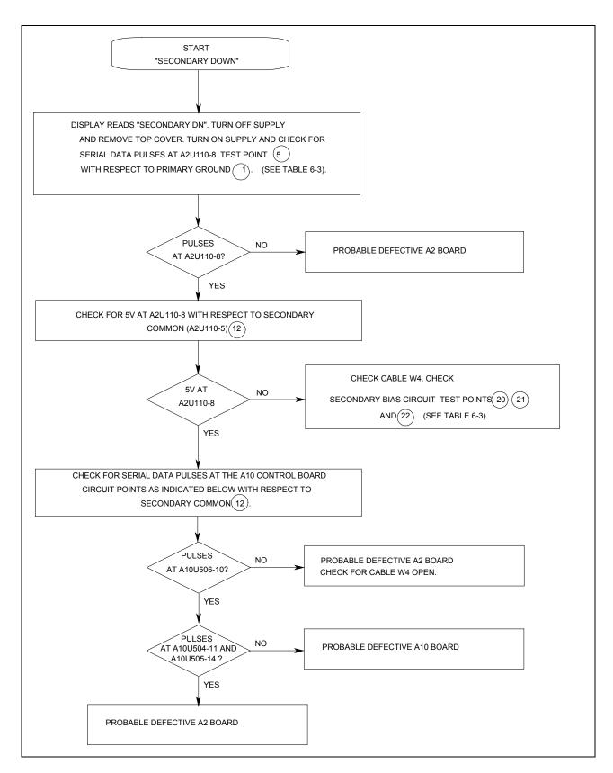
Figure 3-9. Secondary Interface Down)
