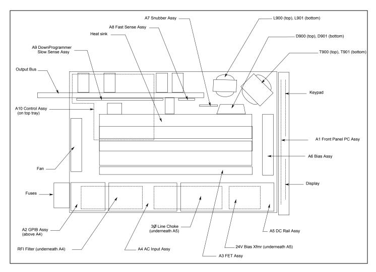
Figure 3-14. Component Locations (Top Cover and RFI Shield Removed)
