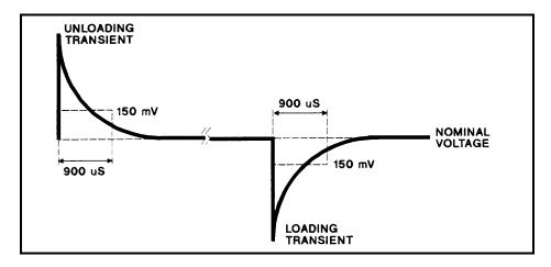
Figure 2-2. Transient Response Waveform
