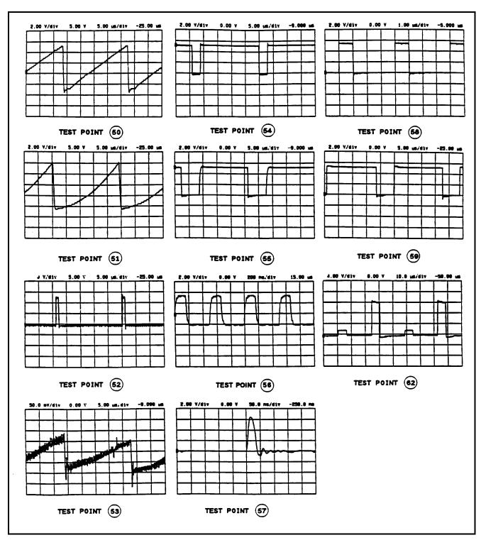
Figure 6-1. Test Point Waveforms for Table 6-3 (sheet 2 of 2)
