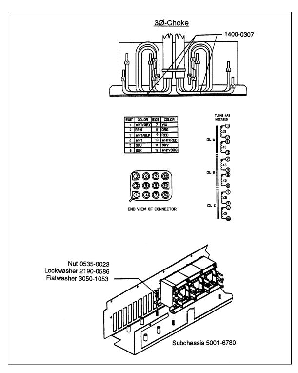
Figure 3-19. Three-Phase Line Choke Subchassis Wiring
