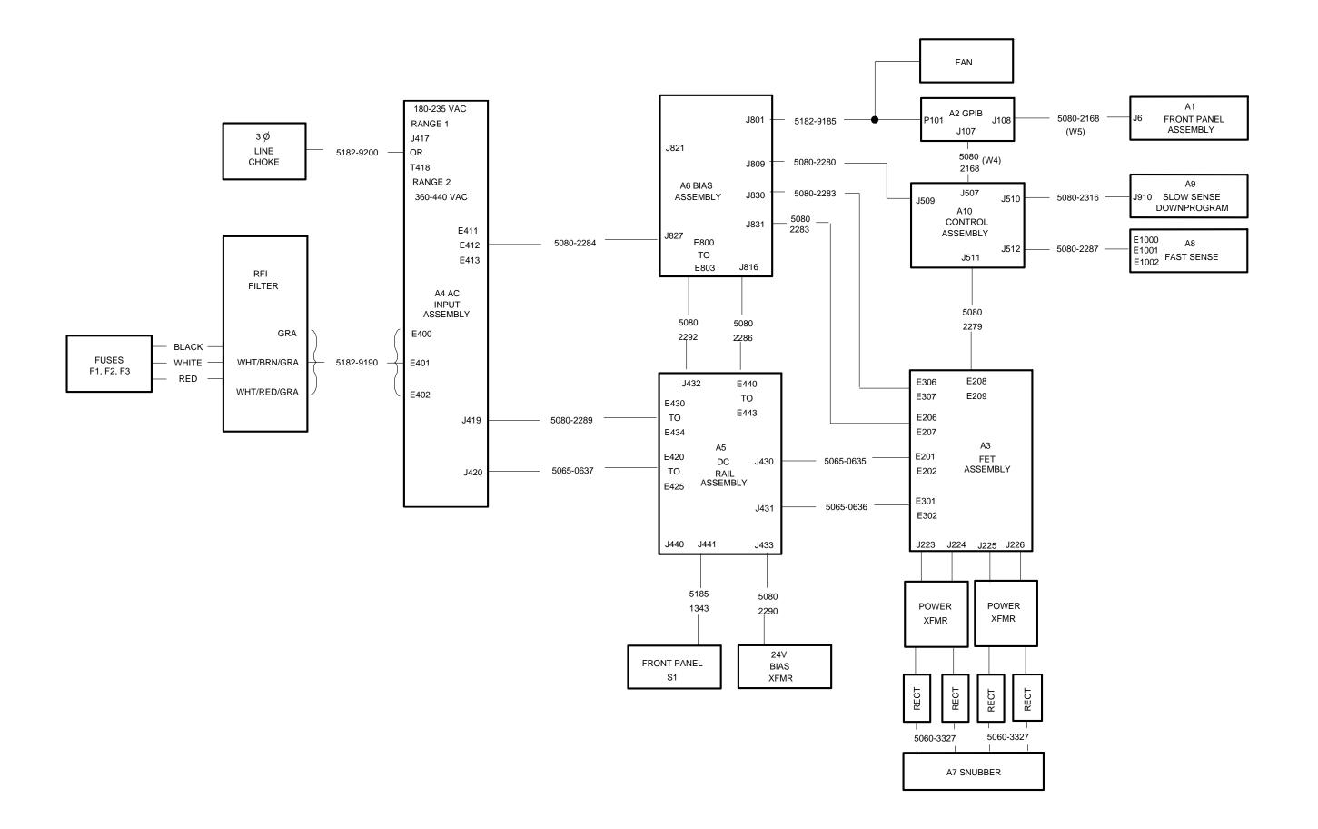
Figure 6-2. Circuit Board Cabling Diagram
