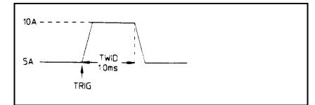
Figure 5-6. Pulsed Transient Operation
