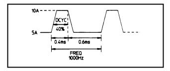
Figure 5-5. Continuous Transient Operation
