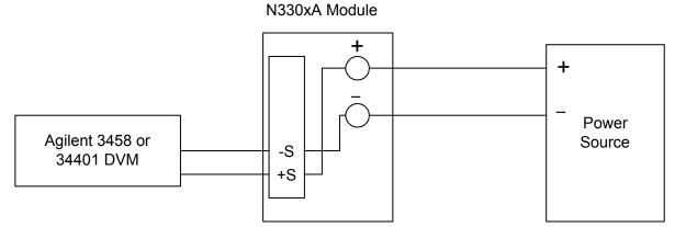
Be sure sense switch is in RMT position
