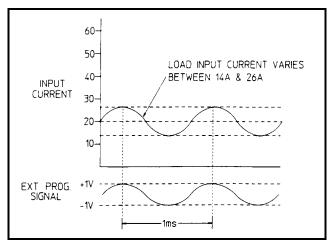
Figure 2-9. External Programming Example
