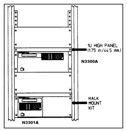
Figure 3-4. Rack Installation
