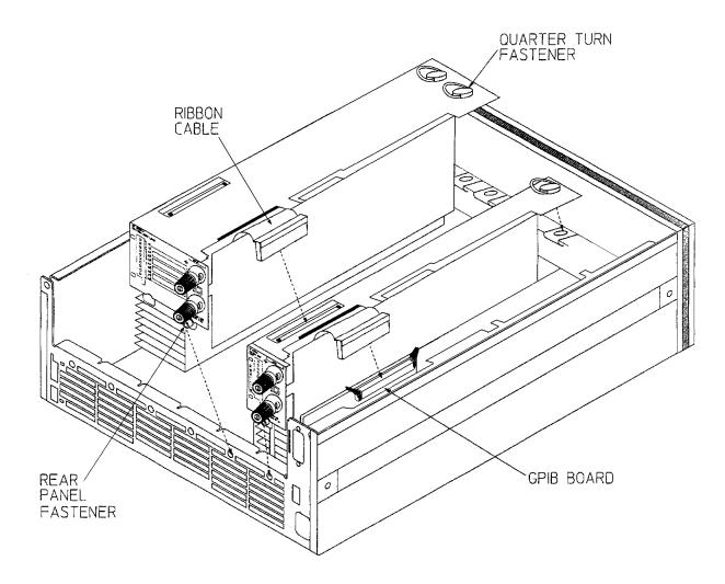
Figure 3-1. Module Installation Diagram
