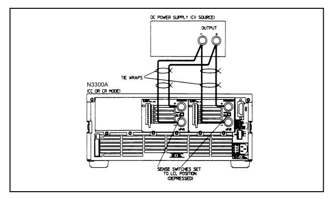
Figure 3-12. Parallel Operation
