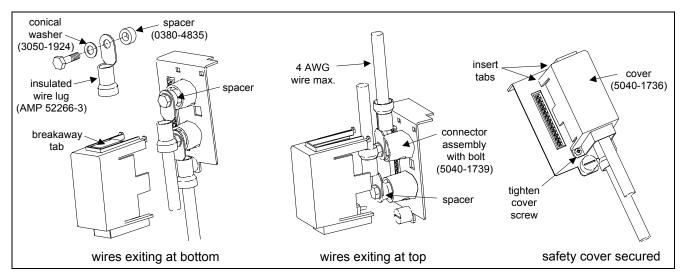
Figure 3-6b. 8mm Screw Terminal Connectors
