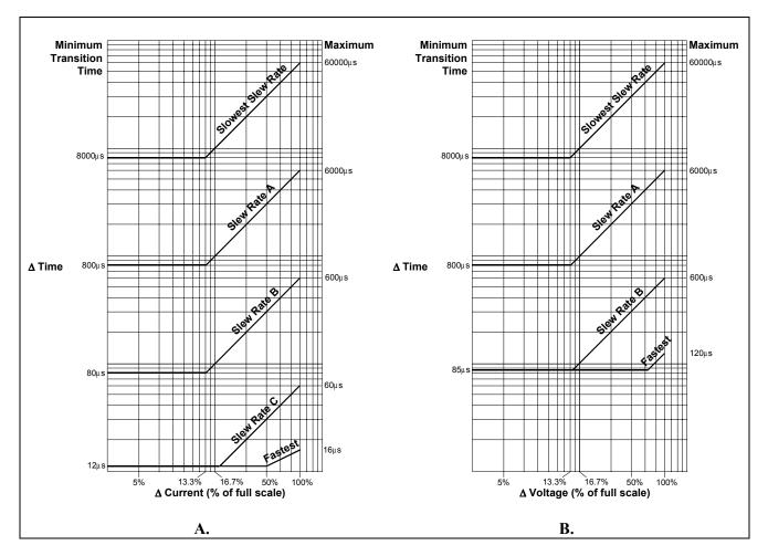
Figure 2-8. Transition Time Slew Rate Examples
