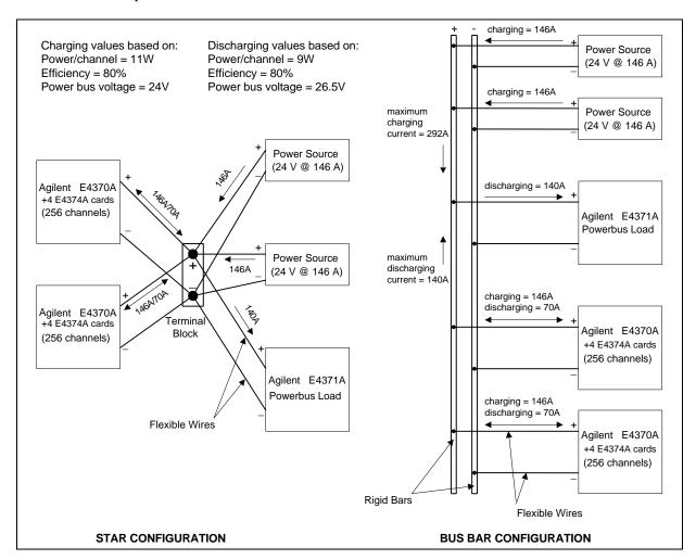
Figure 2-1. Typical Power Bus Configuration for Agilent E4374A cards
