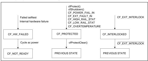
Figure 5-4. Instrument Protect States
