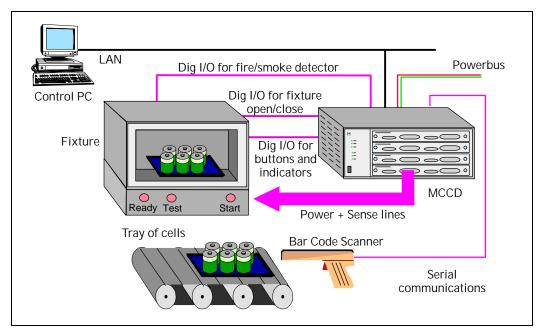
Figure 1-7. Typical Cell Forming Station
