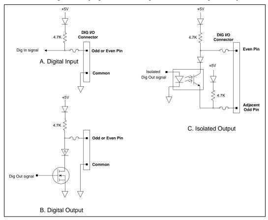
Figure 2-3. Equivalent Digital I/O Circuits
