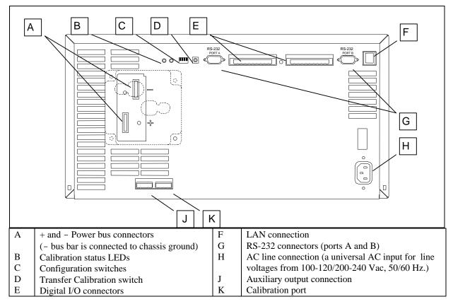
Figure 1-3. Agilent E4370A MCCD Mainframe Rear Panel Connections
