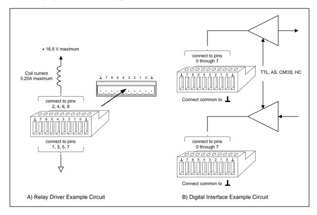
Figure 2-4. Typical Hardware Connections
