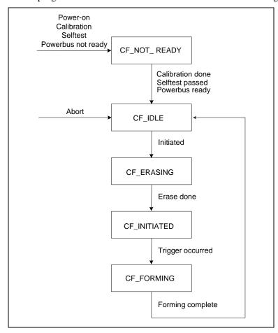
Figure 5-3. Instrument Run State
