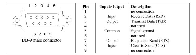
Figure 2-5. RS-232 A and B Connectors
