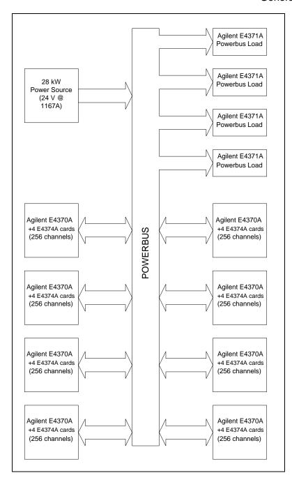
Figure 1-5. System Diagram Using Agilent E4374A Cards
