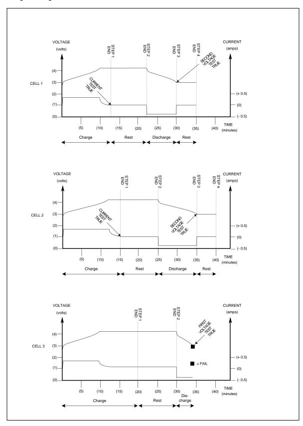
Figure 5-2. Simple Cell Forming Example
