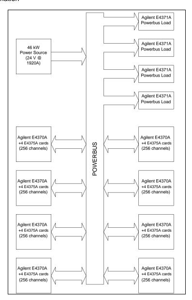
Figure 1-6. System Diagram Using Agilent E4375A Cards
