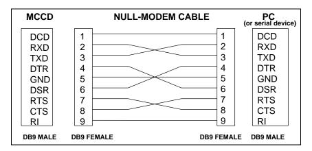
Figure 2-6. Null-modem Cable Connections
