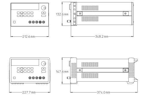
Figure 8-1. Dimensions of Agilent E3632A Power Supply
