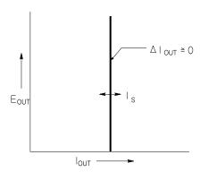
Figure 7-3. Ideal Constant Voltage Power Supply
