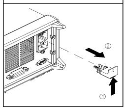
2 *Install the correct line fuse.* Remove the power-line voltage selector from the power-line module.
