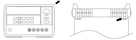
To remove the rubber bumper, stretch a corner and then slide it off.
