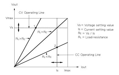
Figure 7-5. Output Characteristics
