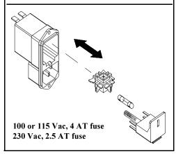
**3** Rotate the power-line voltage selector until the correct voltage appears.
