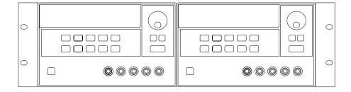
To rack mount two instruments of the same depth side-by-side, order link kit 5061-9694 and flange kit 5063-9214.
