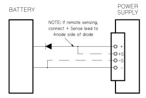
Figure 3-1. Recommended Protection Circuit for Battery Charging
