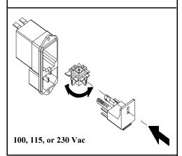
4 Replace the power-line voltage selector and the fuse-holder assembly in the rear panel.
