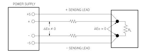
Figure 7-7. Regulated Power Supply with Remote Sensing
