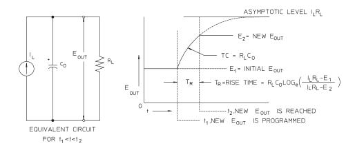
Figure 7-8. Speed of Response - Programming Up (Full Load)
