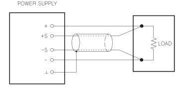
Figure 3-2. Remote Voltage Sensing Connections
