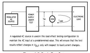
Figure A-7. Basic Test Setup
