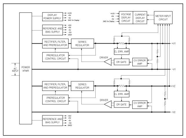
Figure A-1. Block Diagram
