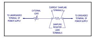
Figure A-5. Current Sampling Resistor Connections
