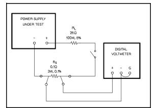
Figure A-6. Output Current, Test Set Up
