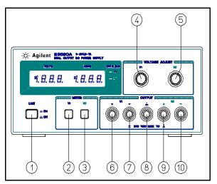
**Figure 2. Front-Panel Controls and Indicators**
