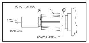
**Figure A-4. Front Panel Terminal Connections**
