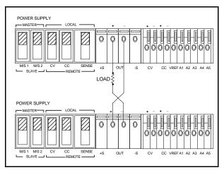
Figure 11. Normal Series Operation of Two Supplies
