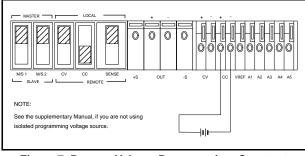
Figure 7. Remote Voltage Programming, Constant Current
