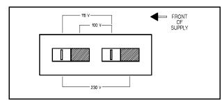
Figure 2. Line Voltage Selector (set for 115 Vac)
