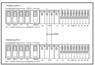
Figure 8. Normal Parallel Operation of Two Supplies
