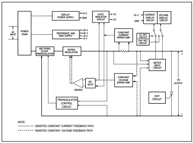
Figure A-1. Block Diagram
