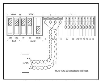
Figure 5. Remote Voltage Sensing
