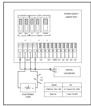
Figure A-4. Basic Test Setup
