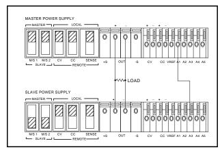
Figure 9. Auto-Parallel Operation of Two Supplies
