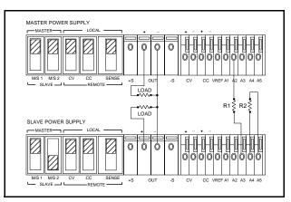
Figure 14. Auto-Tracking Operation of Two Supplies
