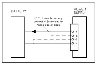
Figure 17. Recommended Protection Circuit for Battery Charging
