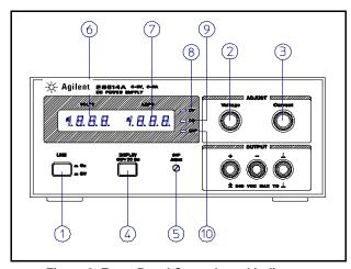
Figure 3. Front-Panel Controls and Indicators
