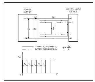
Figure 16. Reverse Current Loading Solution
