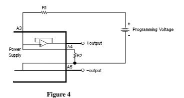
The output will always be the same or less than the programming voltage. The M/S2 switch must be in the down position. For best results, place a  $0.1\mu F$  capacitor in parallel with R2.
