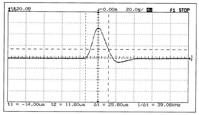
Figure A-5. Load Transient Response Time Waveform
