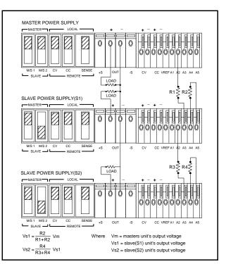
Figure 15. Auto-Tracking Operation of Three Supplies
