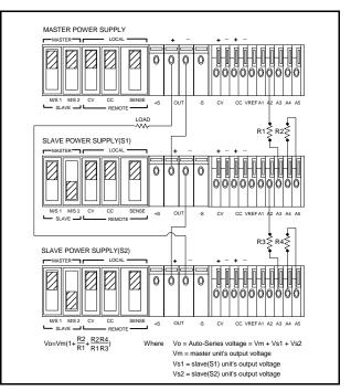
Figure 13. Auto-Series Operation of Three Supplies
