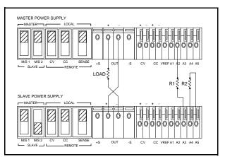
Figure 12. Auto-Series Operation of Two Supplies
