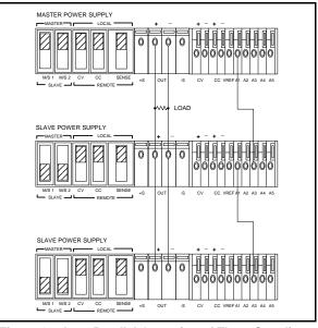
Figure 10. Auto-Parallel Operation of Three Supplies
