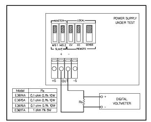
Figure A-9. Calibration Test Setup
