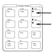
The following chart shows the commands in the Voltage function menu. Some commands may not appear on all models. Menus are circular, you can return to the starting position by continuously pressing  $\triangle$  or  $\nabla$ .
