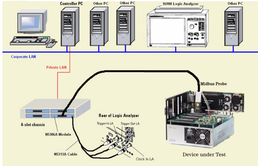
This diagram illustrates the basic external protocol analyzer connection. The protocol analyzer's controller PC is connected to the corporate LAN and has a second LAN card for creating a private LAN between the controller PC and one or more protocol analyzer chassis. The logic analysis system must be connected to the same corporate LAN as the controller PC.
