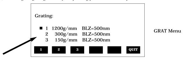
This menu shows that Grating #1 (1200g/mm, blazed at 500nm) is in the operating position. To select grating #2, press the white button under the number 2 on the display. During the 20 seconds required for a grating change, the controller displays "Changing Grating". When the change is complete, the dot (■) appears next to the #2 grating. To return back to the Main Menu, press the white key below the QUIT function. The Main Menu will now display the new grating.
