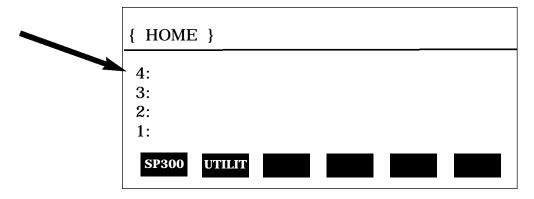
If the above menu **does not** appear (for example, if the controller was operated in the calculator mode), press the RIGHT FUNCTION KEY (¬), followed by the LIBRARY key, then select SP300. When the above menu is displayed, press the white key below the **SP300** function to begin operation (see Appendices Section for use of the "UTILIT" functions). The following menu will be shown:
