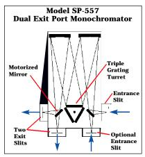
Includes micrometer controlled dual exit slits (90 & 180°), and motorized mirror for rapid, computer controlled exit slit selection.
