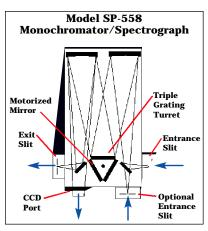
Includes dual exit ports; one exit slit and one sliding tube CCD adapter with motorized mirror for rapid, computer controlled exit port selection.
