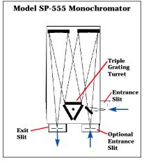
Includes  $90^{\circ}$  optical path, and micrometer adjustable entrance and exit slits.
