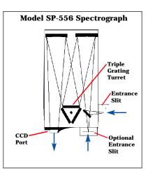
Includes 90° optical path, large 14mm X 27mm focal plane, plus sliding tube CCD adapter with focus-stop.
