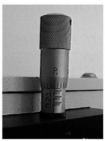
Slit Width Setting: 200 Micrometers (0.200mm)
