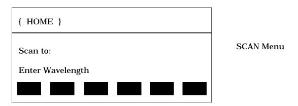
As with GOTO, key in the desired wavelength (in nm) followed by <ENTER>. The SpectraPro-500i will scan to the selected wavelength at the preset scanning rate. To change the scanning rate, see the **SPEED** (**Scanning Rate**) instructions following this section. The controller will continue to update the wavelength display as scanning takes place. When the scanning is complete, the controller returns to the Main Menu with updated information:
