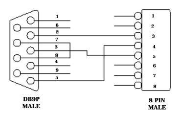
SpectraPro-500i to Macintosh Computer (Modem or Printer Port)
