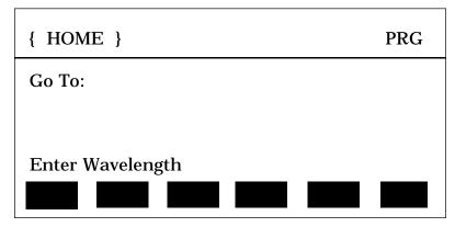
Key in the desired wavelength (in nm) and then push the <ENTER> key (ex: 500 <ENTER>). The SpectraPro-500i will then race at the maximum motor speed to the selected wavelength and display this interim menu.
