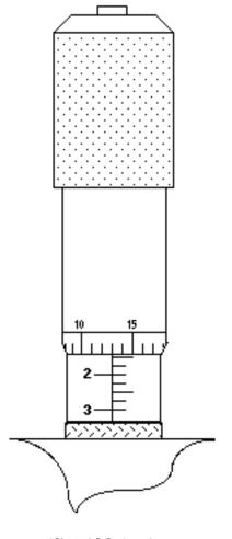
Slit Width Setting: 1380 Micrometers (1.38mm)
