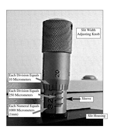
Slit Width Setting: 200 Micrometers (0.200mm)
