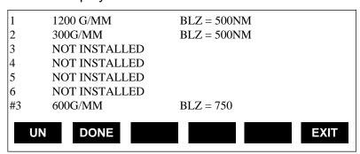
Select DONE to install the grating as displayed on the line directly above the labels. Select UN to un-install the grating specified on the line directly above the labels. Select EXIT to return to the utilities menu if neither of these selections were made. Selecting INST from the utilities menu followed by the NXT key and then selecting EXIT allows checking the gratings installed without making any changes.
