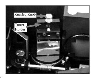
Dual Grating Turret Mounted Inside the SpectraPro-150
