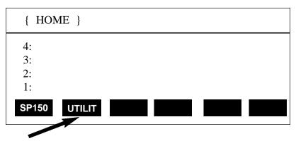
If the above menu **does not** appear (for example, if the controller was operated in the calculator mode), press the RIGHT FUNCTION KEY ( $\Rightarrow$ ), followed by the LIBRARY key, then select SP150. When the above menu is displayed, press the white key below the **UTILIT** function to access the utilities. The following menu will be shown:
