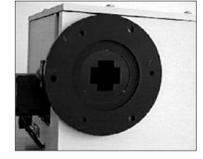
Array Detector Mounting Flange Mounted in Place of the Exit Slit
