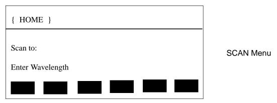
As with GOTO, key in the desired wavelength (in nm) followed by <ENTER>. The SpectraPro-150 will scan to the selected wavelength at the preset scanning rate. To change the scanning rate, see the **SPEED (Scanning Rate)** instructions following this section. The controller will continue to update the wavelength display as scanning takes place. When the scanning is complete, the controller returns to the Main Menu with updated information:
