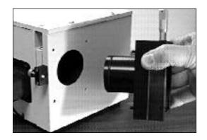
Sliding the Exit Slit Assembly, With Sliding
