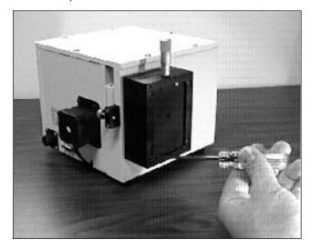
Removal of the 8-32 Screws Securing the Exit Slit to the SpectraPro-150 Housing
