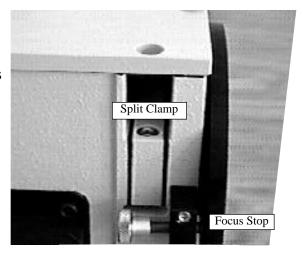
8. If fibers or other imaging input optics are used to bring light into the SpectraPro-150, they will require adjustment along the optical axis to achieve best vertical image quality.
