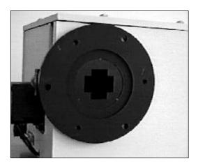
Standard Array Detector Mounting Flange
