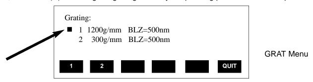
This menu shows that Grating #1 (1200g/mm, blazed at 500nm) is in the operating position. To select grating #2, press the white button under the number 2 on the display. During the 20 seconds required for a grating change, the controller displays "Changing Grating". When the change is complete, the dot (■) appears next to the #2 grating. To return back to the Main Menu, press the white key below the QUIT function. The Main Menu will now display the new grating.
