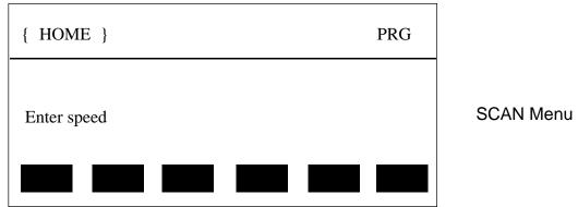
Key in the desired scanning speed in nm/min then press <ENTER> (ex: 200.0 <ENTER>). If you enter a wavelength above the maximum scanning speed for a specific grating, the SP-150 and controller will default to the maximum scanning speed allowed for the specific grating. The controller will return to the Main Menu with updated scan speed, as shown in the menu below:
