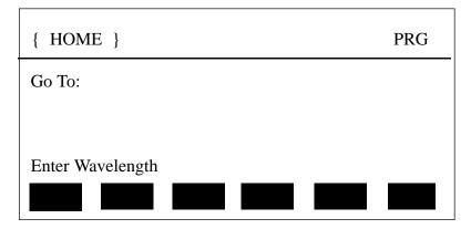
Key in the desired wavelength (in nm) and then push the <ENTER> key (ex: 500 <ENTER>). The SpectraPro-150 will then run at the maximum motor speed to the selected wavelength and display this interim menu.
