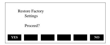
Selecting YES will restore all grating parameters and default initialization settings to the original factory settings. This process takes approximately 20 seconds. Note that any gratings that were installed since receiving the SP-150 will be eliminated from memory and must be re-installed. Selecting NO will make no changes to memory.
